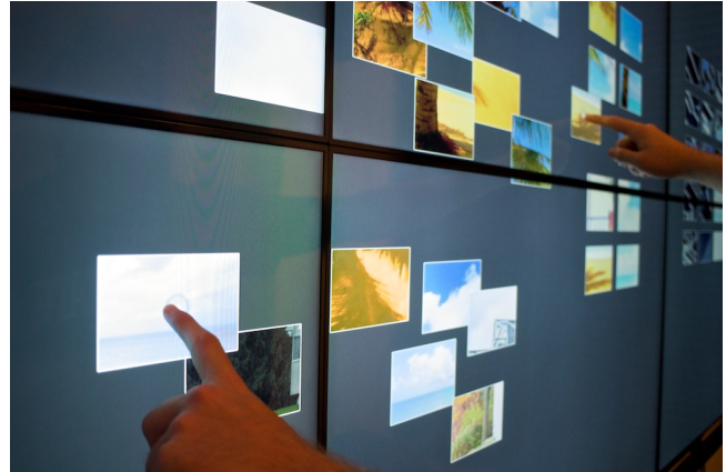
Figure 1: Tiling many independent displays provides a means of creating large workspaces that can support activities such as data visualization and sensemaking, but introduces interior bezels.
