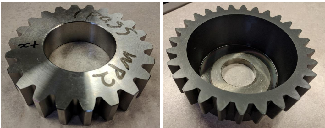
Figure 4.18: Finished workpiece (left) and tool (right) for external spur gear case study.
