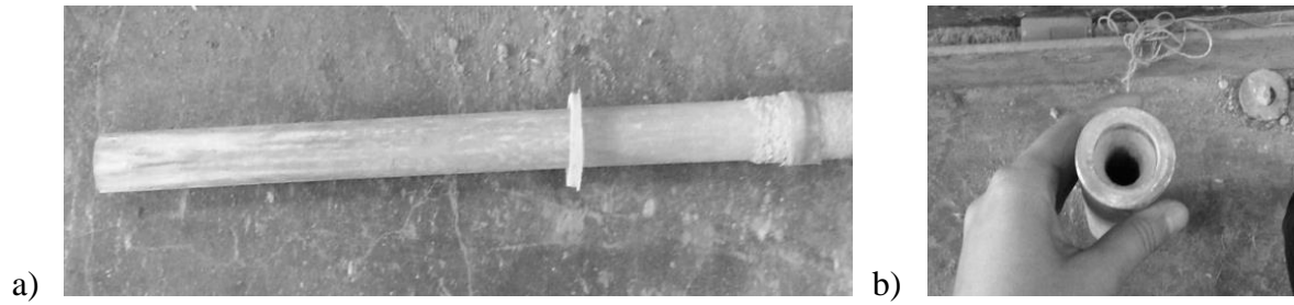
Fig. 4.3 – Company I bars’ anchorage failure a) bar view, b) tube view
