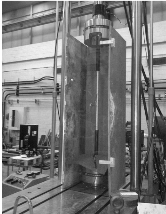
Fig. 4.1 – a) Anchorage system for tensile test specimen, b) tension test in progress
