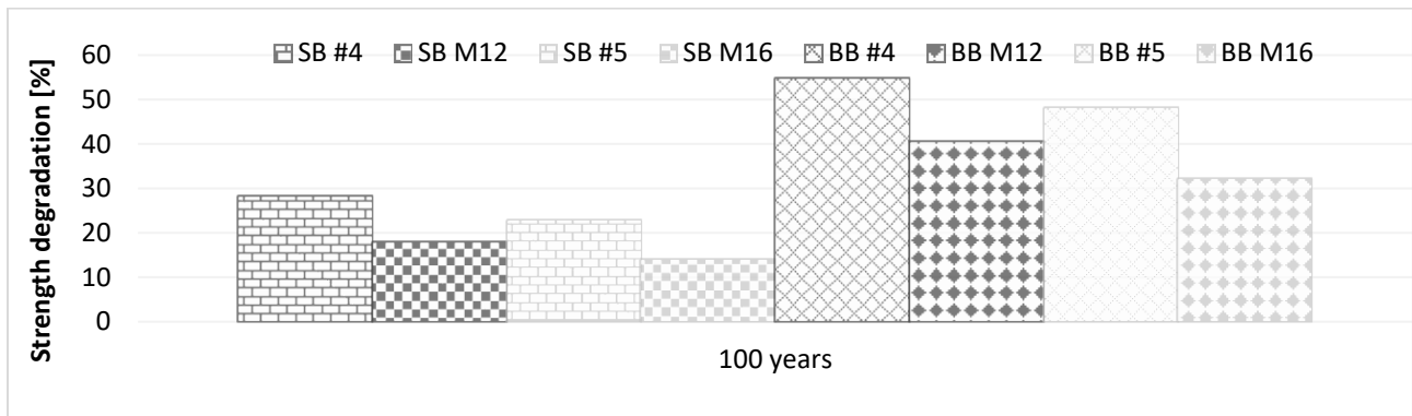
Fig. 7.30 – Results comparison for flexure strength degradation after 100 years of use
