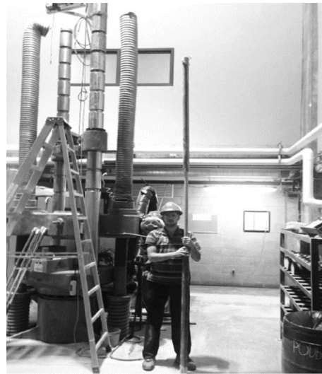
Fig. 4.18 – Tensile test sample for 25 mm bar diameter from Company I (Sherbrook University – Benmokrane 2014)
