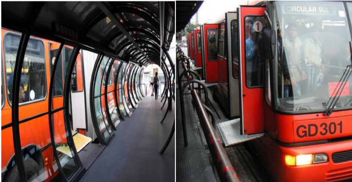
Figure 10 Curitiba's bus boarding tubes. Left, the interior of downtown multi-bus tubes look and function like a metro station; right, downtown bus tubes support five-door boarding, and a folding ramp allows same-level boarding and alighting. (Jian, 2010; Karis, B. et al., 2006)
