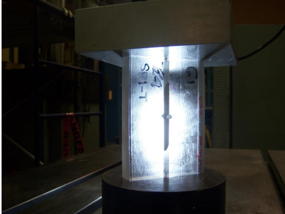
Figure 20: Photo taken at 175kN and 6.82mm compressive displacement respectively. The upper arm fracture propagated to 40 mm and the lower arm fracture propagated to 37mm. Both arms show tunneling and their shape show mirror symmetry about the center hole. The upper arm has moved towards the front face while the lower arm has moved towards the rear face.
