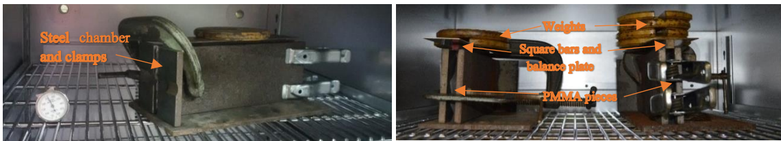
Figure 2: Compression chamber within the oven to create thermal bonding. Stress is applied normal to the thickness of the sample by the dead weight. Temperature is held at 150°C (300°F) and it is confirmed by the interior thermostat for 6 hours. Above, 12.7 mm (0.5 in) thick sample scenario 1 being bonded at high temperature. Below, 24.5 mm (1 in) thick sample scenarios 4 (left) and 5 (right) cooling down after 6 hours of cooking.
