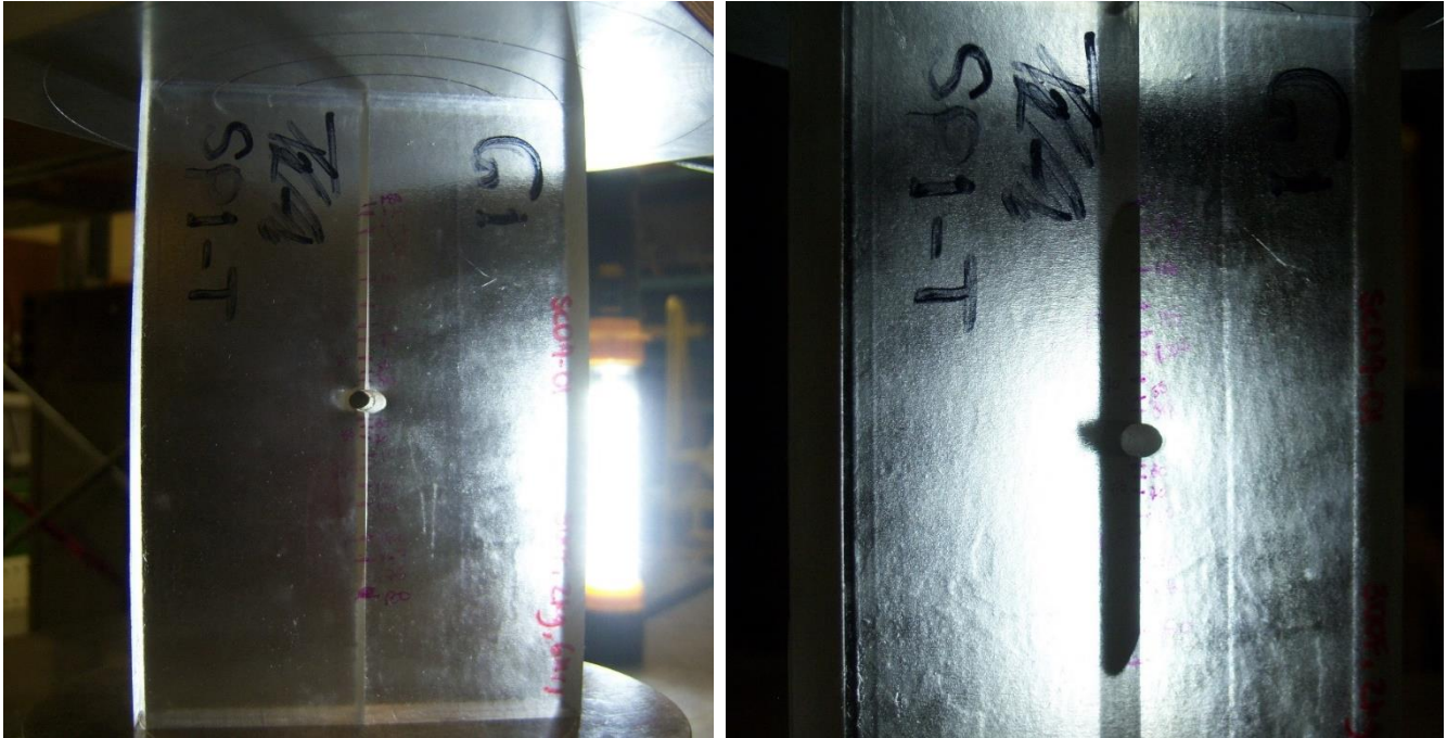
Figure 22: Left, front face of rectangular specimen at 180kN uniaxial compression force. The center hole has deformed from a drilled circle to an oval from the large load it sustains. At the vertex of the center hole and the interface, some small gap is visible, this is considered the fracture aperture. On the right, there is a close view of the fracture geometry. The measurement for all specimens is taken at the maximum extension of the fracture and not an average.
