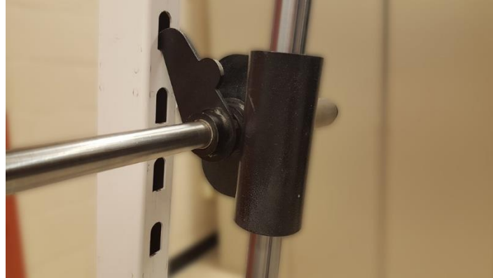
Figure 7. Locking hooks installed on either side of the barbell.
