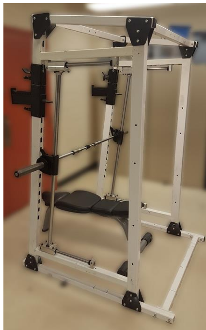
Figure 3. Modified Smith machine allowing for coupled anterior-posterior translation and uncoupled medial-lateral translation.
