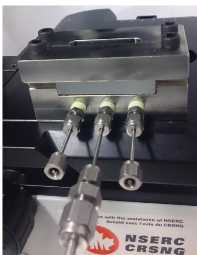
Figure A.2 A close look at the assembly of connector/microchip.
