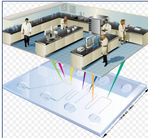
Figure 1.1. Example of components of Lab-on-a-chip platform for carrying out multiple tasks (top image)[7]. Schematic description of miniaturization of traditional laboratory processes onto an integrated Lab-on-a-chip device (bottom image)[1].
