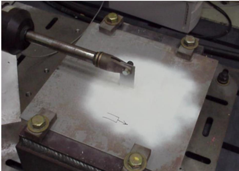
Figure 5-3: Test sample of the T-joint subjected to in-plane cyclic loading (JD)
