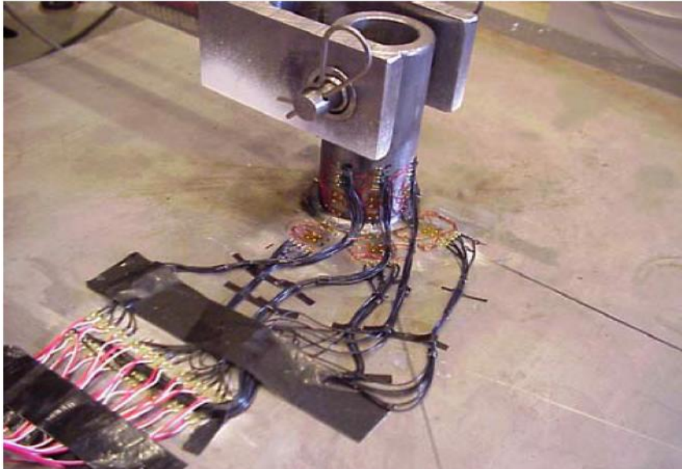
Figure 5-39: JD experiment for the tube-on-plate welded joint subjected to lateral loading (JD)
