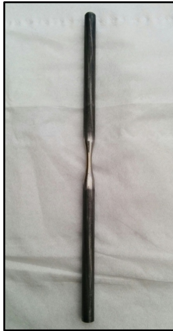
Figure 3.17: Specimen machined from centre 7-wire strand
