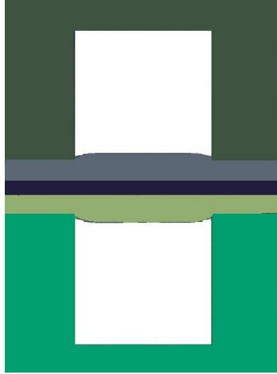
Figure 4-8 A schematic drawing of a single PEM fuel cell channel with deformation
