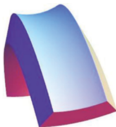
Figure 3.2: Deformation of an LCE with twisted-nematic texture showing saddle-like bending. Figure taken from [63].
