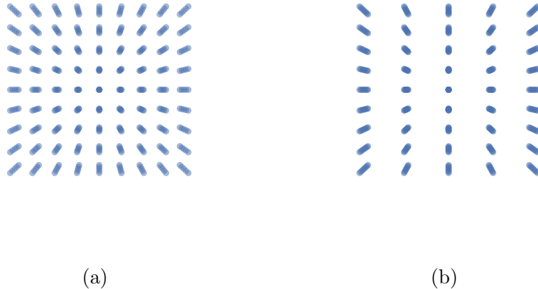
Figure 2.1: Atoms in a simple tetragonal lattice viewed (a) along and (b) perpendicular to the unique axis.
