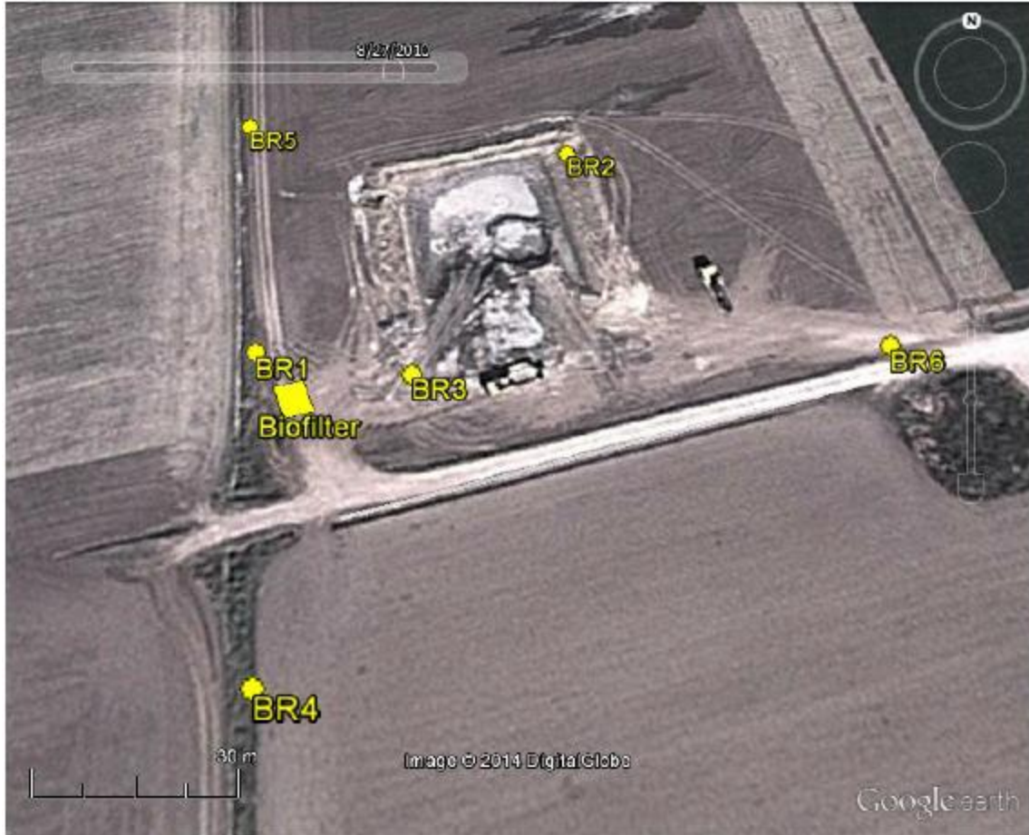
Figure 5.2 Keswick (tile drain) site: Map of the site with the locations of the biofilter and monitoring well bundles BR1 through BR6.
