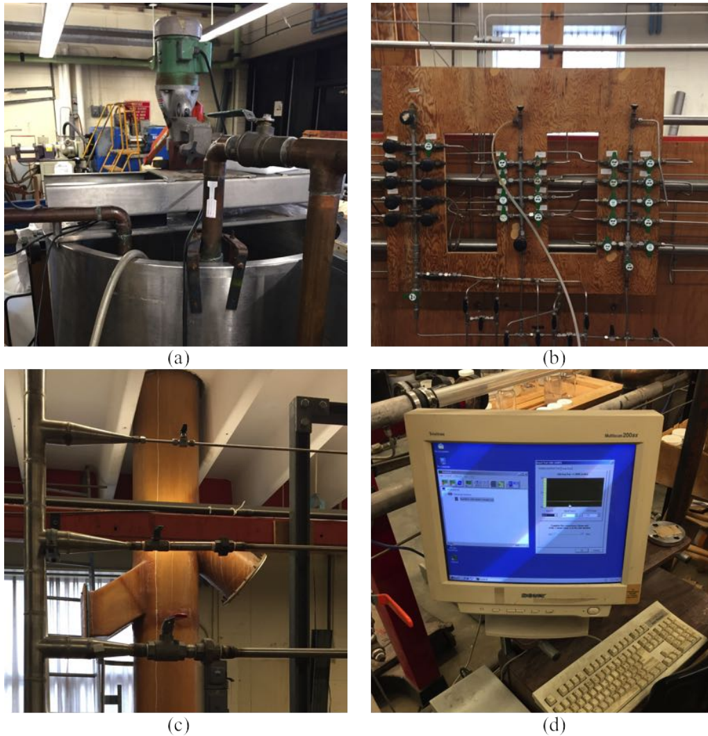
Figure 2-2 Photos of pipeline flow loop set-up: (a) the mixing tank; (b) the control panel; (c) different size pipelines, from top to bottom is 0.5 inch, 1.0 inch and 1.5 inch; (d) the computer terminal of data acquisition system.
