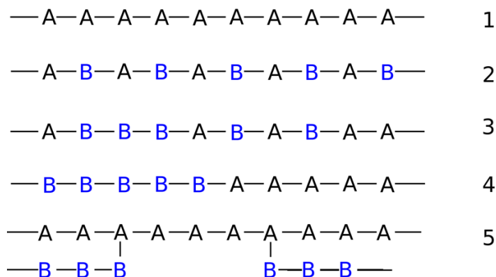
Figure 1: Different classes of copolymers. 1) Homo-polymer. 2) Alternating copolymer. 3) Random copolymer. 4) Block copolymer. 5) Graft polymer.
