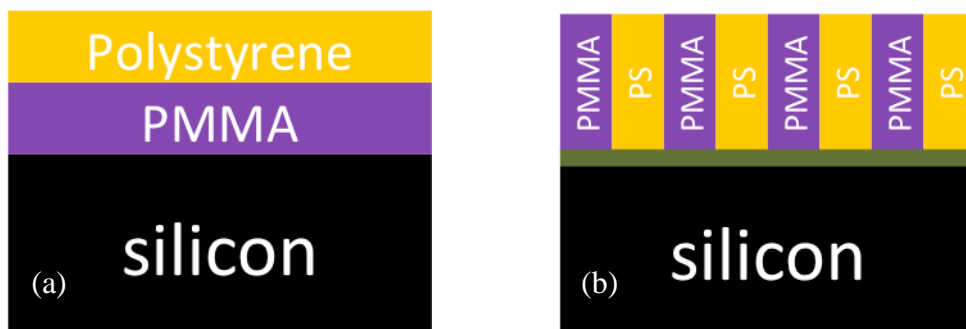
Figure 51: a) Horizontal self-assembled lamella on a non-neutralized silicon surface. b) Vertical self-assembled lamella on a neutralized silicon surface (the green area represents 3-MPTS monolayer).
