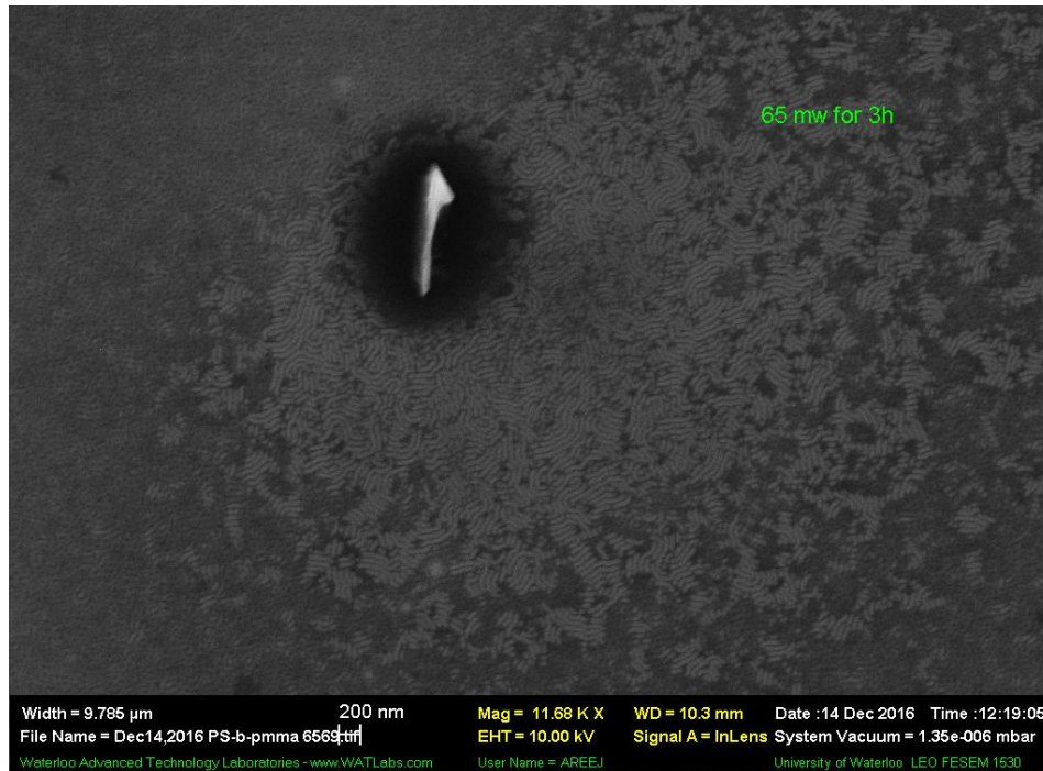
Figure 26: SEM image of annealed BCP 65 at 190 °C for 3 hours.
