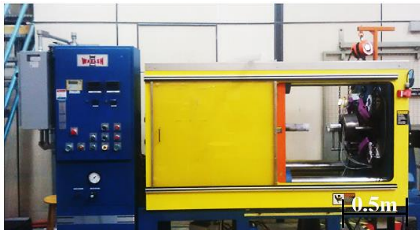
Figure 4.7: Wabash laboratory scale extruder used for strip extrusion of AA6xxx alloys
