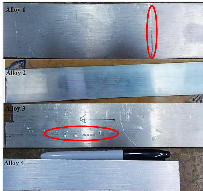
Figure 5.21: Surface quality of alloys 1 – 4 after laboratory scale extrusion at 500 °C
