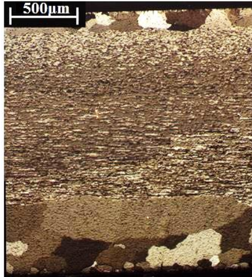
Figure 5.30: Surface to surface microstructure of alloy 3 (500 ^{\circ}\text{C} )
