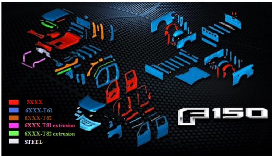
Figure 1.4: Frame of F150 showing parts manufactured with processed aluminum [10]
