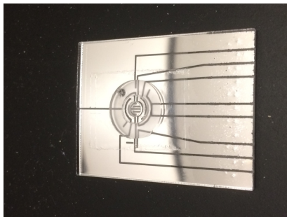
Figure 2.1: Image of a complete chip from PMMA side of the chip. The well and moat are visible in the center with heater traces protruding to the right. The sensor is located directly below the well and is obscured in this image. Electrical contact is made to the right edge of the chip using a zero insertion force (ZIF) socket (TE Connectivity 2-531020-8-ND, Digikey).
