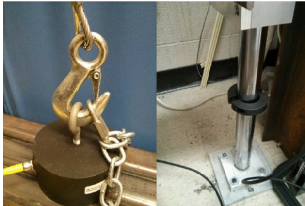
FigureA 11: Left is the safety chain which wraps around the load carriage and connects to the winch hook in case the electromagnet fails; Right are adjustable shaft collars which attach to the drop tower's vertical shaft
