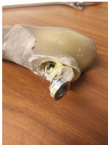
FigureA 14: Uncoiling of the threaded insert, and surrounding area on the proximal femur
