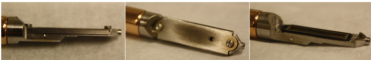
Figure 4.7: The holder prototype manufactured by HTC , shown with and without the lid. Note that before use in a TEM , a sapphire bullet would be added, and the screws would be countersunk (i.e. not protruding). The small circular feature visible in the left and right photos is level with the end of the inlet channel.
