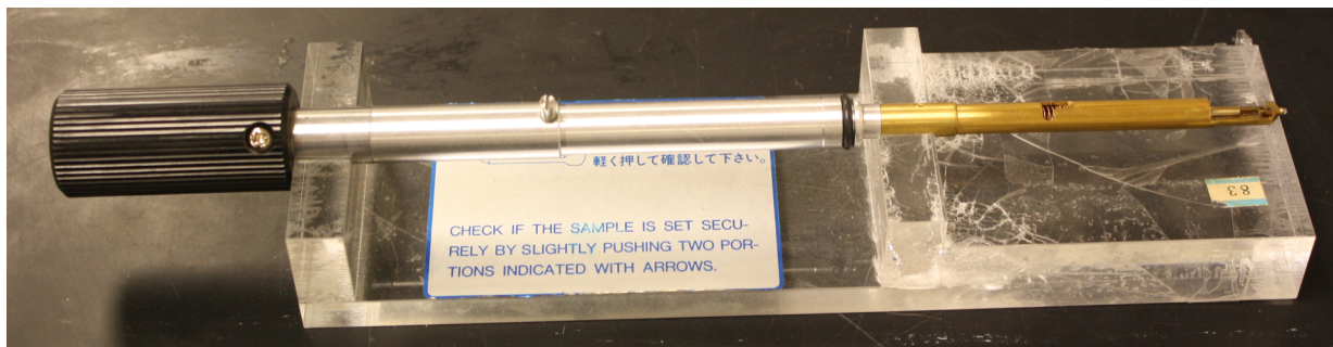
Figure 2.1: A basic Hitachi sample holder (for bulk samples with the HD2000 STEM in scanning mode) used as the basis for the fluidic holder design.
