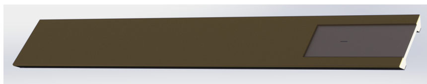
Figure 4.4: Render of the top chip, with a metal spacer. Note how the spacer covers the majority of the chip; this is simpler to produce than a spacer covering only the edges.
