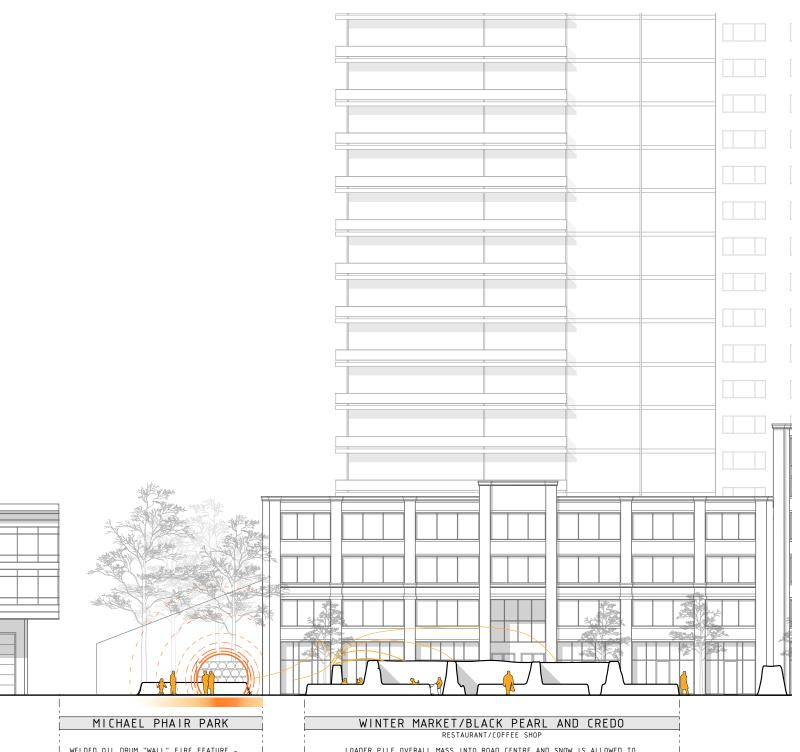
WELDED OIL DRUM "WALL" FIRE FEATURE -CAN BE USED AS LARGE SCALE HEAT SOURCE OR RADIANT COOKING SYSTEM. FURNISHINGS CONSTRUCTED BY BOBCAT AND SHOVEL
