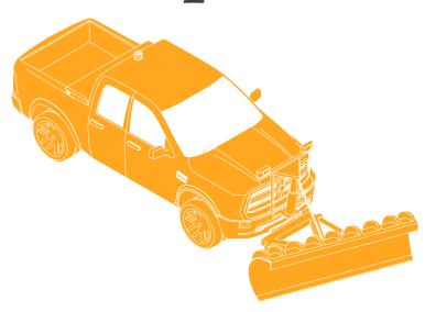
A mainstay of private snow removal companies yet still available to the Public Works vehicle fleet, the snow plough attachment on a pickup is a lower scale version of a full road maintenance vehicle. The pickup can be deployed to areas too small/restrictive for heavier equipment, and does not require transportation like a Bobcat or snowblower.
