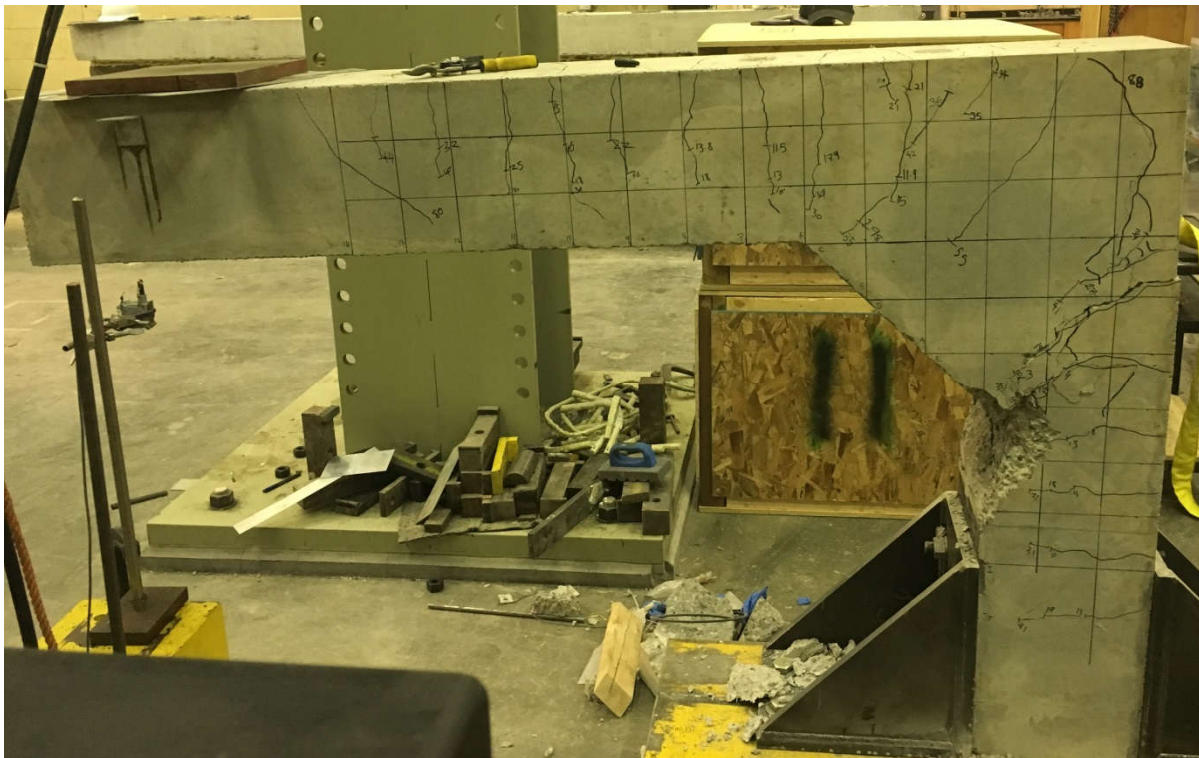
Figure 4.24: Crack Patterns on East Face, CB-3-6
