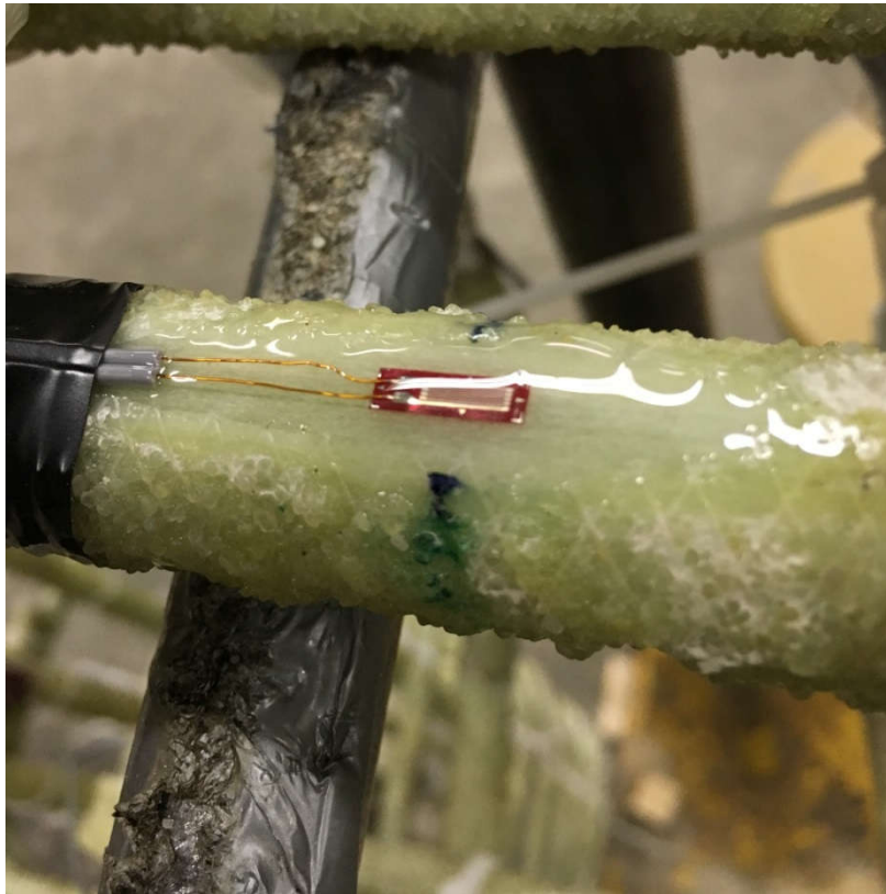
Figure 3.15: Installed Strain Gauge
