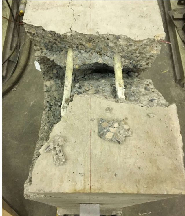
Figure A.51: Top View of UA-2-4, Showing Spalling on One Side
