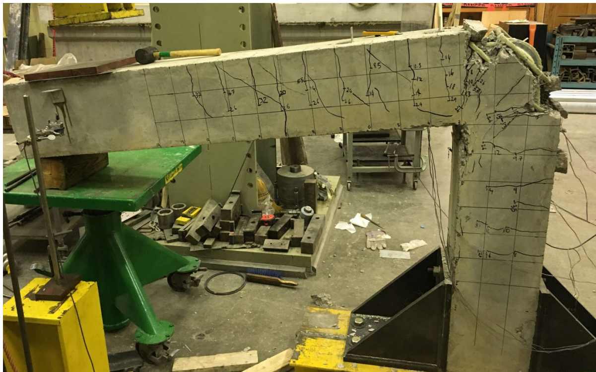
Figure 4.19: Crack Patterns on East Face, CA-3-6
