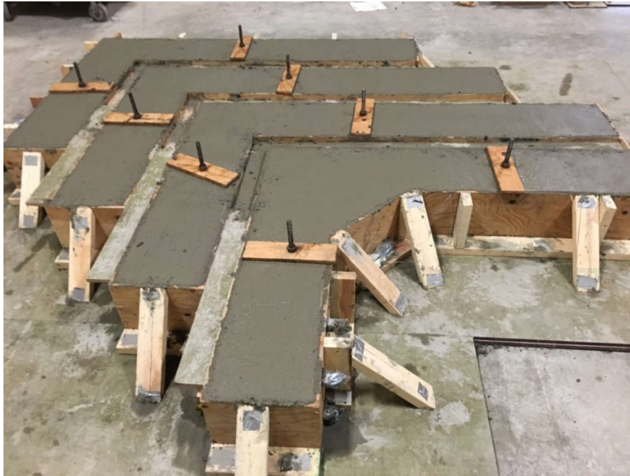
Figure 3.11: Poured Specimens with Anchors Installed
