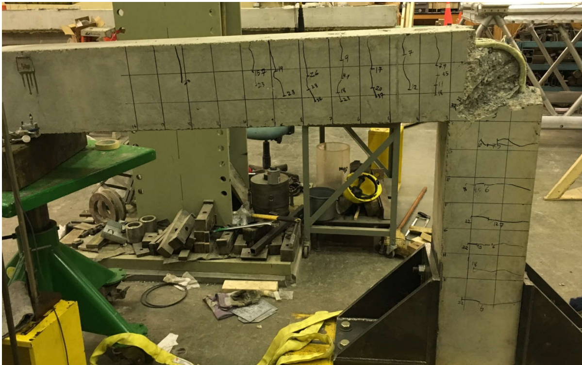
Figure 4.11: Cracking Patterns on East Face, UA-3-6
