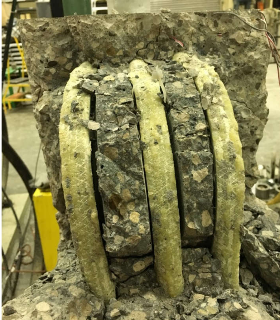
Figure A.21: North Side of Failed Joint, UA-3-6
