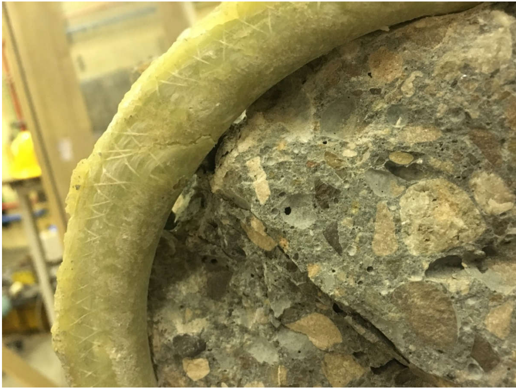
Figure A.14: Crack in Bent Portion with Waving Also Visible, UA-4-6
