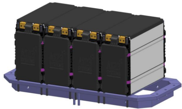
Figure 72: Lower Mounting Section of ESS
