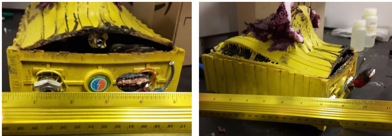
Figure 55: Post-mortem analysis first assessment of thermal runaway
