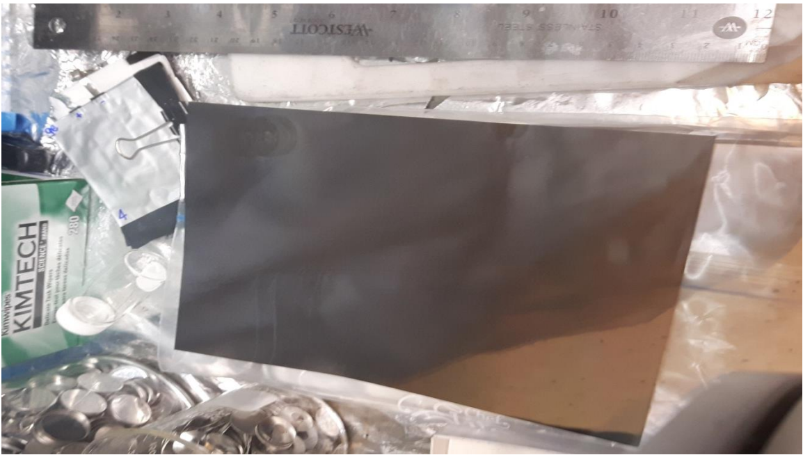
Figure 97: LFP electrode aged 35°C 100% SOC
