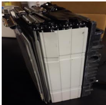
Figure 3: Cross-Section of De-Constructed A123 Battery Pack
