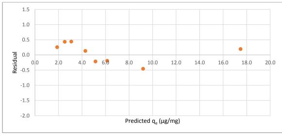
Figure A.26 Residual plot for equilibrium isotherm of CYL adsorption by the BG-HHM (wood)
