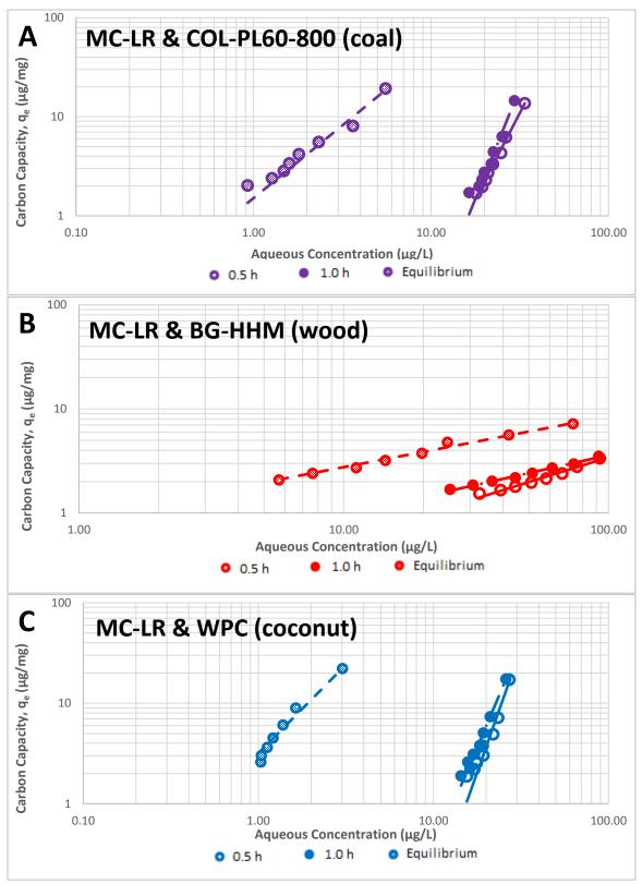
Figure A.50 Freundlich model plot demonstrating PAC adsorption of ANTA at contact time of 0.5 h, 1 h and equilibrium (straight lines showing Freundlich fitting curves and symbols showing experimental data). A) Coal-based PAC; B) wood-based PAC; C) coconut-based PAC.
