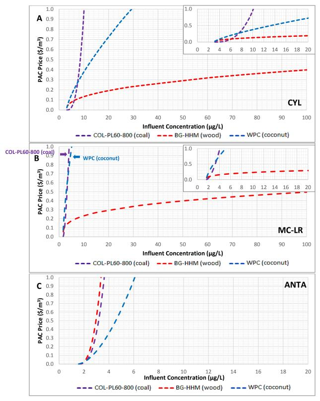
Figure 4.10 Estimate of PAC costs for adsorption of cyanotoxins at given range of influent concentrations in Lake Erie water, based on SEBCM under 0.5 h non-equilibrium conditions, given a target cyanotoxin concentration of 1.5  $\mu$ g/L. A) CYL, B) MC-LR, C) ANTA
