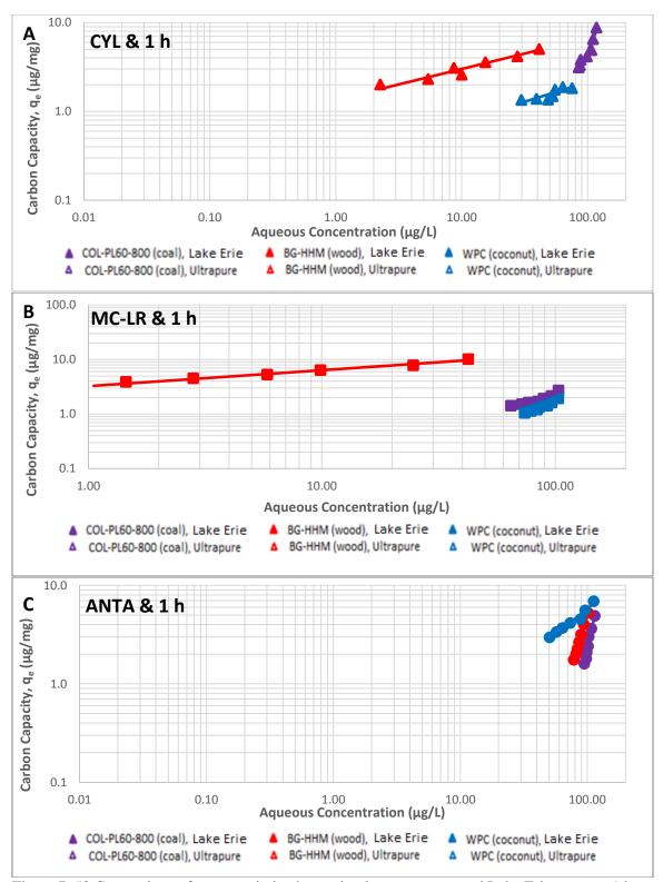
Figure B.50 Comparison of cyanotoxin isotherms in ultrapure water and Lake Erie water at 1 h. A) CYL, B) MC-LR, and C) ANTA
