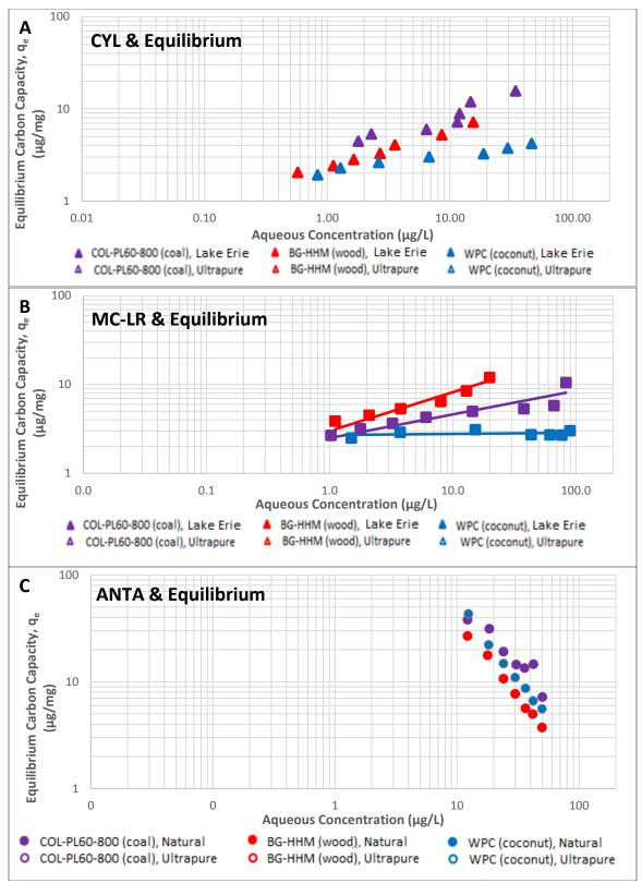
Figure B.51 Comparison of cyanotoxin isotherms in ultrapure and Lake Erie water at equilibrium. A) CYL, B) MC-LR, and C) ANTA
