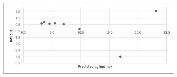
Figure B.47 Residual plot for the equilibrium isotherm of ANTA adsorption by the WPC (coconut)
