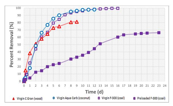
Figure 5.1 CYL removal in ultrapure water by virgin and preloaded GACs as a function of time; initial CYL concentration =  $100 \mu g/L$ , GAC dose = 50 mg/L.
