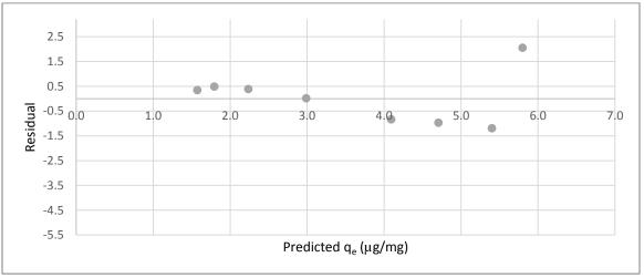
Figure B.29 Residual plot for the equilibrium isotherm of CYL adsorption by the WPC (coconut)
