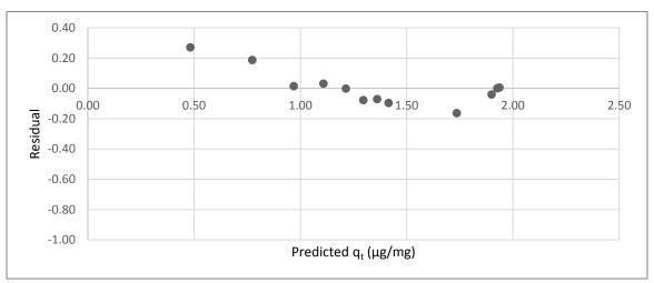
Figure A.20 Residual plot for pseudo-second order fit of ANTA adsorption by the WPC (coconut)
