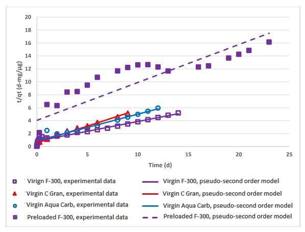
Figure 5.2 Pseudo-second order kinetic model fits using virgin and preloaded GACs in ultrapure water
