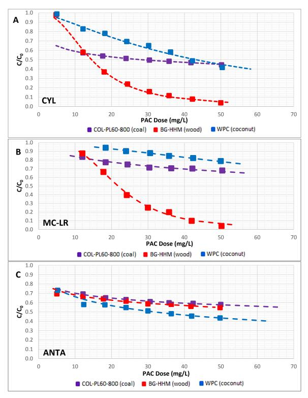
Figure 4.8 Cyanotoxin adsorption in the presence of NOM in Lake Erie water using coal-, wood-, and coconut-based PACs, based on the 0.5 h non-equilibrium data. A) CYL adsorption, B) MC-LR adsorption, C) ANTA adsorption
