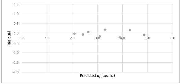
Figure A.27 Residual plot for 0.5 h isotherm of CYL adsorption by the WPC (coconut)
