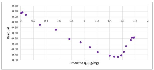
Figure C.9 Residual plot for pseudo-first order fit of CYL adsorption by the pre-loaded F-300 (coal)
