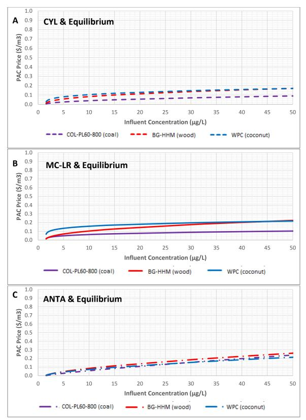
Figure B.78 Estimate of PAC costs for adsorption of cyanotoxins at influent concentrations in Lake Erie water, based on SEBCM under equilibrium conditions, given target cyanotoxin concentration of  $1.5 \mu g/L$ . A) CYL adsorption, B) MC-LR adsorption, C) ANTA adsorption
