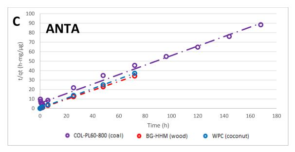
Figure A.11 Pseudo-second order kinetic model fits of cyanotoxin adsorption by three PACs in ultrapure water. A) CYL, B) MC-LR, and C) ANTA.
