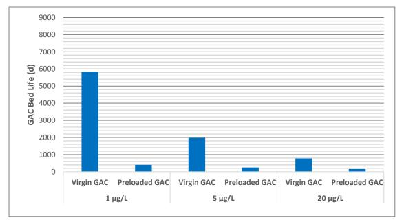
Figure 5.6 ECM predicted GAC bed-life for virgin and preloaded coal-based GAC in a singlesolute system with influent CYL concentrations of 1, 5 and 20 µg/L for an EBCT of 10 min.
