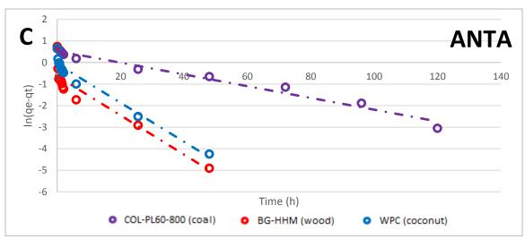
Figure A.1 Pseudo-first order kinetic model fits of cyanotoxin adsorption by three PACs in ultrapure water. A) CYL, B) MC-LR, and C) ANTA.
