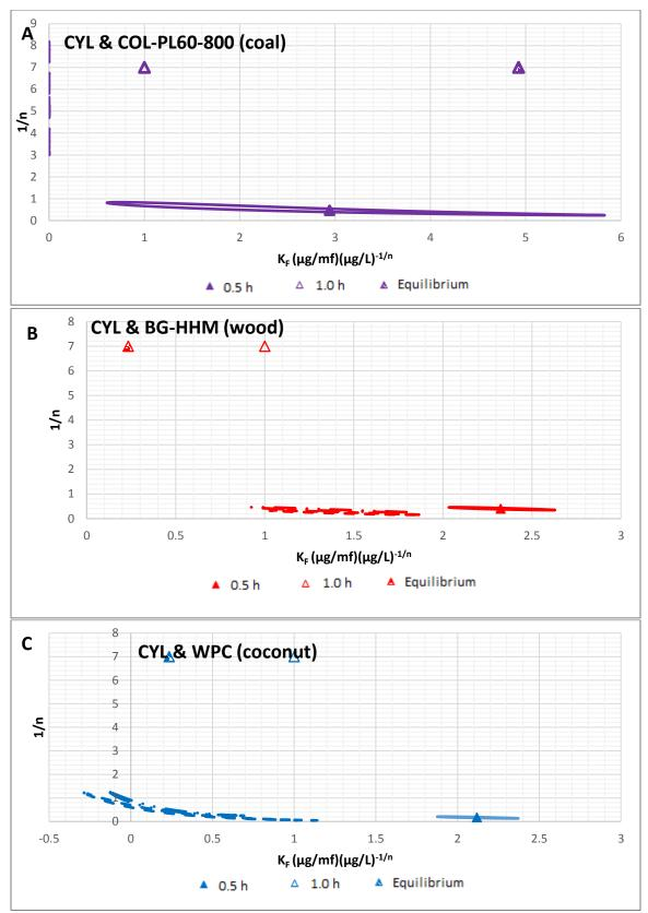
Figure B.48 JCRs of CYL adsorption in Lake Erie water under equilibrium and non-equilibrium conditions, using A) coal-, B) wood-, C) coconut-based PACs
