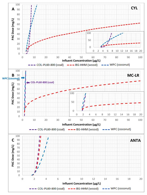
Figure 4.9 Dose estimates for coal-, wood-, and coconut-based PACs for adsorption of A) CYL, B) MC-LR, and C) ANTA in Lake Erie water, based on SEBCM under 0.5 h non-equilibrium condition, given target final concentration of 1.5 µg/L
