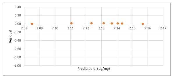
Figure A.13 Residual plot for pseudo-second order fit of CYL adsorption by the BG-HHM (wood)
