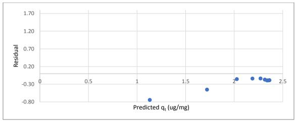
Figure A.2 Residual plot for pseudo-first order fit of CYL adsorption by the COL-PL60-800 (coal)
