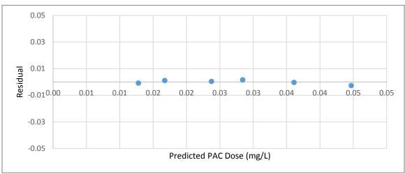
Figure B.68 Residual plot for 1.0 h SEBCM fitting of MC-LR adsorption by the BG-HHM (wood)
