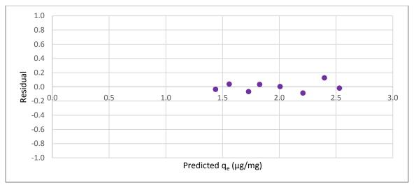
Figure C.13 Residual plot for Freundlich isotherm fitting of CYL adsorption by the pre-loaded F-300 (coal)
