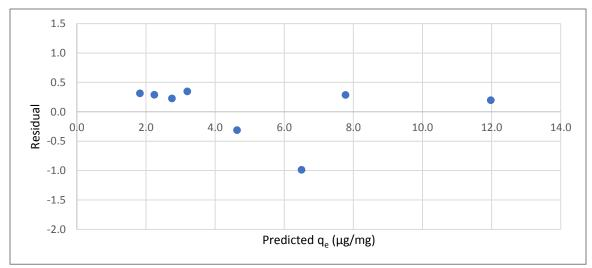
Figure A.23 Residual plot for equilibrium isotherm of CYL adsorption by the COL-PL60-800 (coal)
