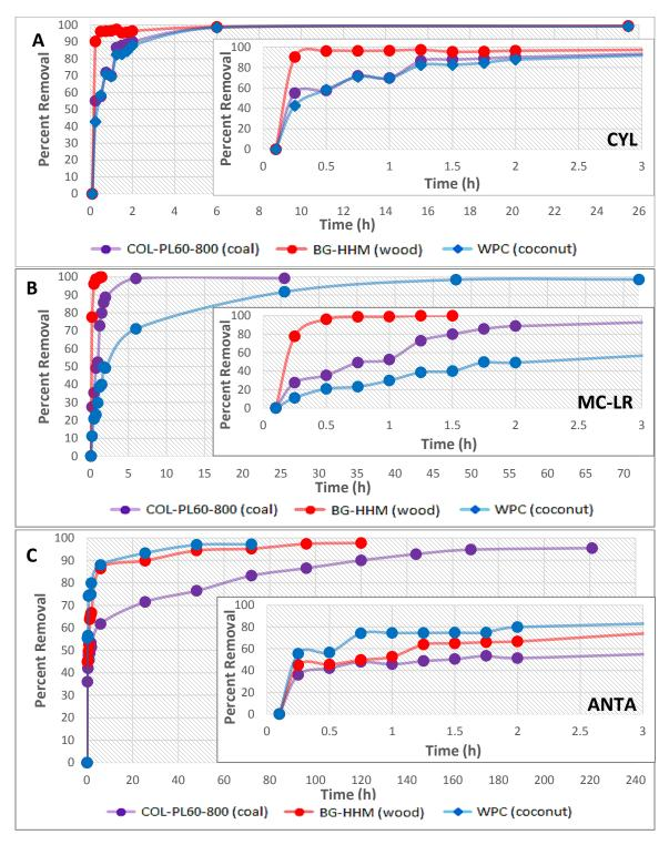
Figure 4.1 Percentage cyanotoxin removal by coal-, wood-, and coconut-based PACs as a function of time: A) CYL removal, B) MC-LR removal, C) ANTA removal.
