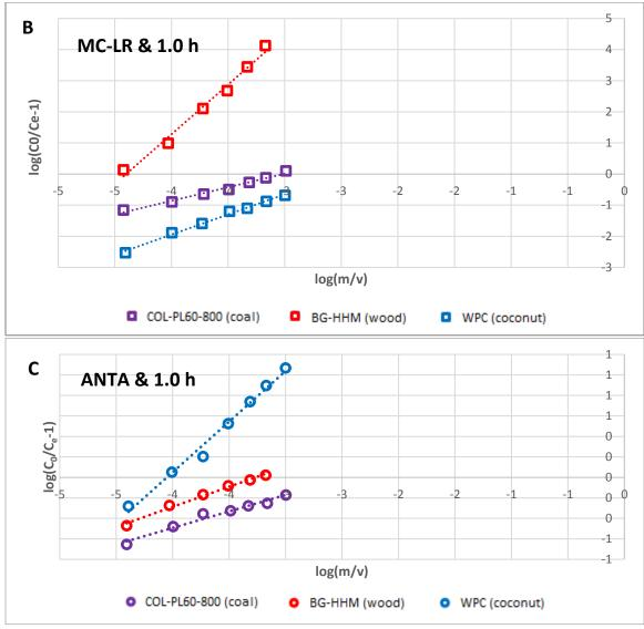
Figure B.62 SEBCM model fitting on the 1h carbon loading data for the adsorption of A) CYL, B) MC-LR, and C) ANTA in Lake Erie water
