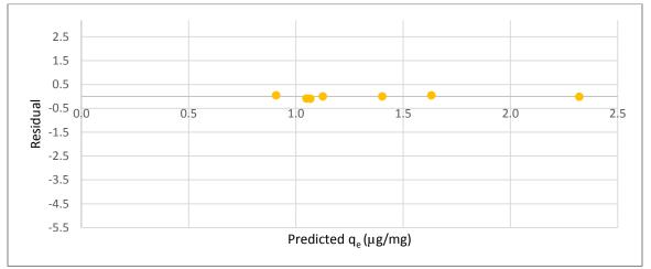
Figure B.30 Residual plot for the 0.5 h isotherm of MC-LR adsorption by the COL-PL60-800 (coal)
