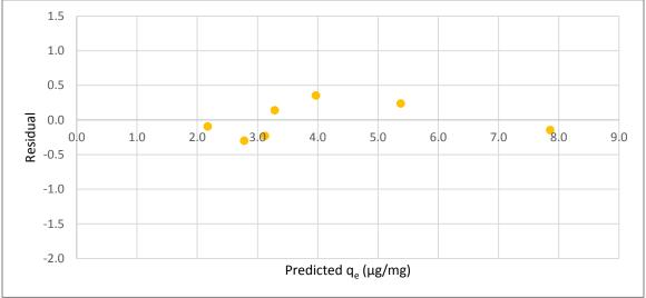
Figure A.32 Residual plot for equilibrium isotherm of MC-LR adsorption by the COL-PL60-800 (coal)
