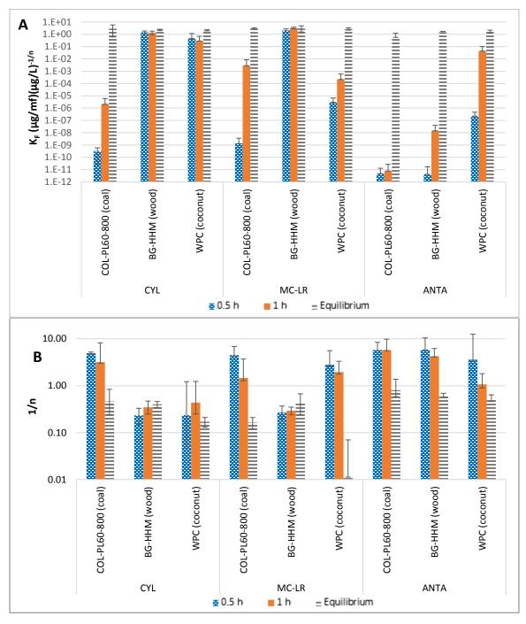
Figure 4.6 Non-linear estimates of Freundlich adsorption parameters with 95% confidence intervals with y-axis in log-scale. A) Freundlich adsorption coefficient (K<sub>F</sub>), B) Freundlich model parameter (1/n)
