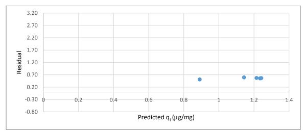
Figure B.16 Residual plot for pseudo-first order fit of MC-LR adsorption by the BG-HHM (wood)
