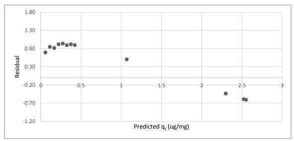
Figure A.10 Residual plot for pseudo-first order fit of ANTA adsorption by the WPC (coconut)
