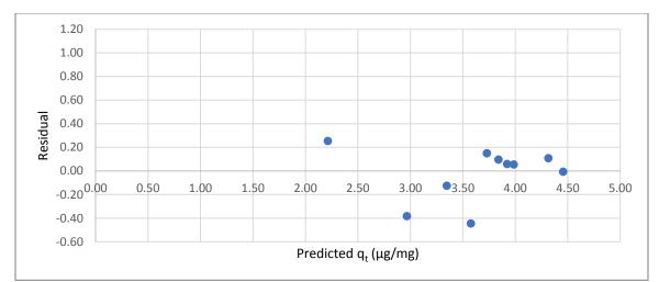
Figure B.2 Residual plot for pseudo-second order fit of CYL adsorption by the COL-PL60-800 (coal)
