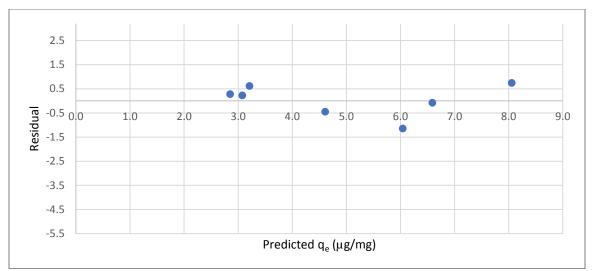
Figure B.22 Residual plot for the 1.0 h isotherm of CYL adsorption by the COL-PL60-800 (coal)
