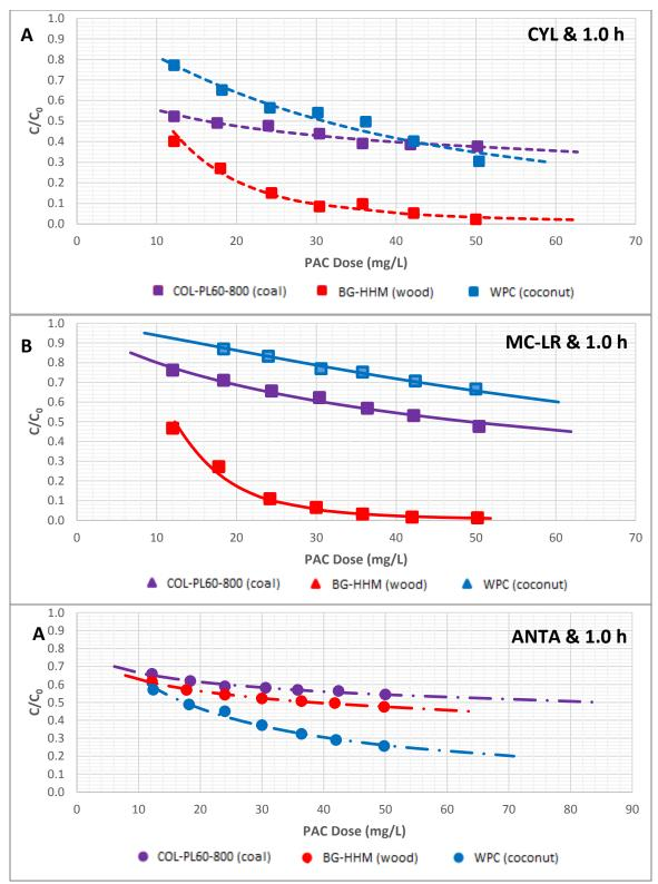
Figure B.63 Cyanotoxin adsorption in the presence of NOM in Lake Erie water using coal-, wood-, and coconut-based PACs, based on the 1 h non-equilibrium data. A) CYL adsorption, B) MC-LR adsorption, C) ANTA adsorption
