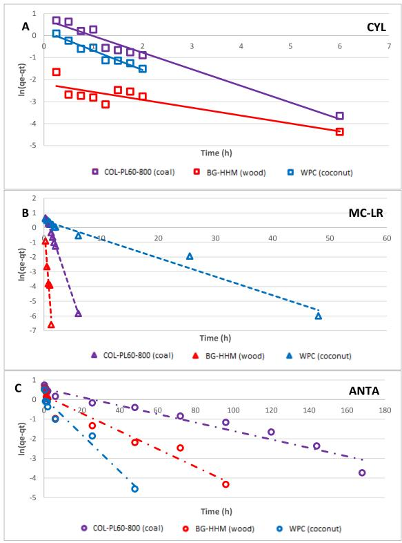
Figure B.11 Pseudo-first order kinetic model fits of CYL, MC-LR, and ANTA adsorption using coal-, wood-, and coconut-based PAC in Lake Erie Water: A) CYL adsorption, B) MC-LR adsorption, and C) ANTA adsorption.
