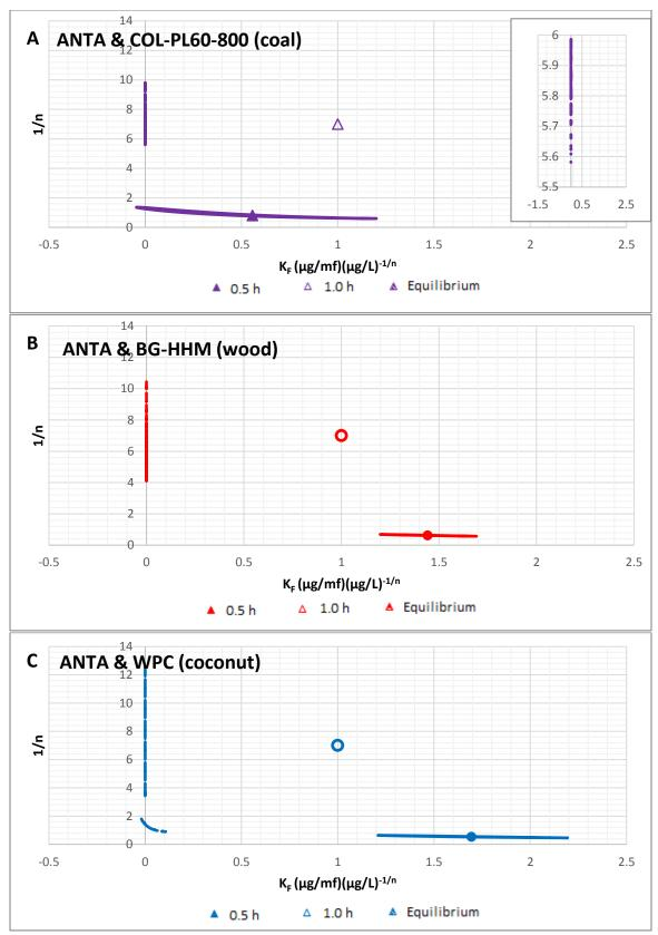
Figure B.49 JCRs of ANTA adsorption in Lake Erie water under equilibrium and non-equilibrium conditions, using A) coal-, B) wood-, C) coconut-based PACs
