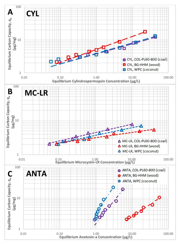
Figure 3.3 Freundlich isotherms for cyanotoxin adsorption by coal-, wood- and coconutbased PACs in ultrapure water. A) CYL, B) MC-LR, C) ANTA. (Straight lines represent Freundlich isotherm model fitting curves and symbols represent experimental data)
