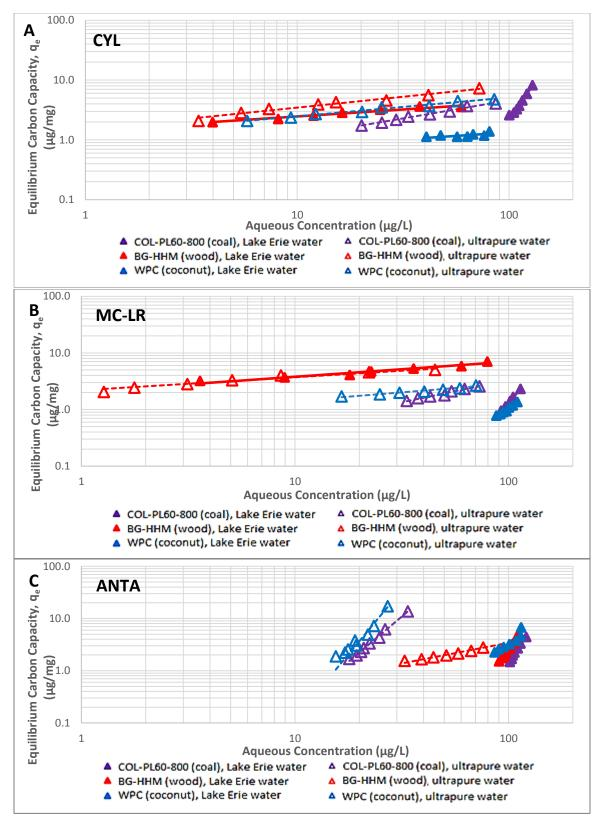
Figure 4.7 Comparison of Freundlich adsorption model fitting for adsorption of three selected PACs for cyanotoxins at 0.5 h contact in both Lake Erie water and ultrapure water. A) CYL adsorption, B) MC-LR adsorption, and C) ANTA adsorption
