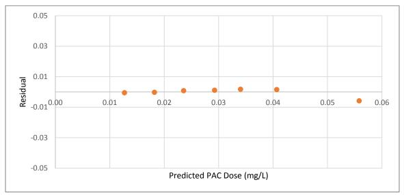
Figure B.54 Residual plot for 0.5 h SEBCM fitting of CYL adsorption by the BG-HHM (wood)
