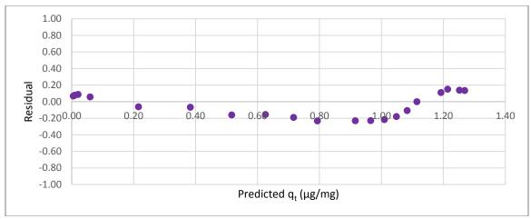
Figure C.4 Residual plot for pseudo-second order fit of CYL adsorption by the pre-loaded F-300 (coal)
