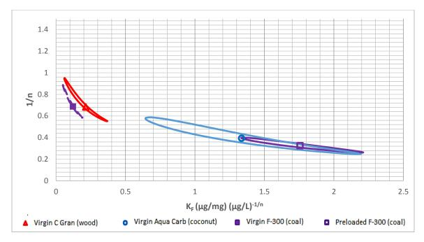
Figure 5.3 The 95% joint confidence region and point estimates for the Freundlich isotherm paramters generated with virgin and preloaded GACs in ultrapure water (ellipses in figure represent JCRs and symbols represent point estimates)
