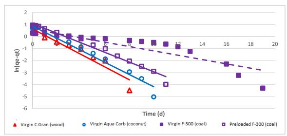
Figure C.5 Pseudo-first order kinetic model fits using virgin and pre-loaded GACs in ultrapure water
