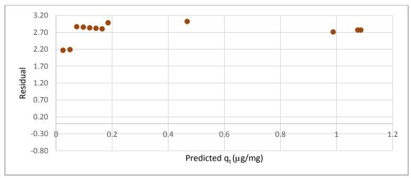
Figure B.20 Residual plot for pseudo-first order fit of ANTA adsorption by the WPC (coconut)
