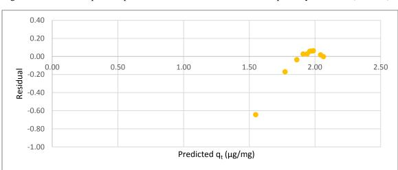
Figure A.14 Residual plot for pseudo-second order fit of CYL adsorption by the WPC (coconut)
