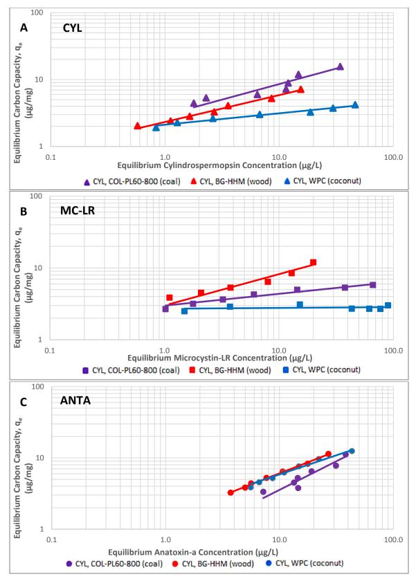
Figure 4.4 Freundlich isotherms for (A) CYL, (B) MC-LR, and (C) ANTA adsorption for coal-, wood-, and coconut-based PACs in Lake Erie water
