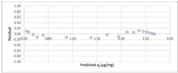
Figure C.1 Residual plot for pseudo-second order fit of CYL adsorption by the virgin F-300 (coal)
