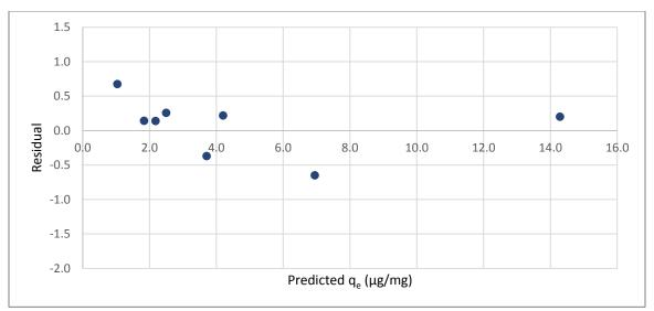
Figure A.40 Residual plot for 1.0 h isotherm of ANTA adsorption by the COL-PL60-800 (coal)
