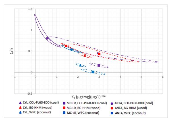
Figure 4.3 95% joint confidence regions and point estimates for CYL, MC-LR, and ANTA adsorption using coal-, wood-, and coconut-based PACs in Lake Erie water at equilibrium (Ellipse curve represents JCR and symbol positioned in the centre of ellipse represents the point estimate)
