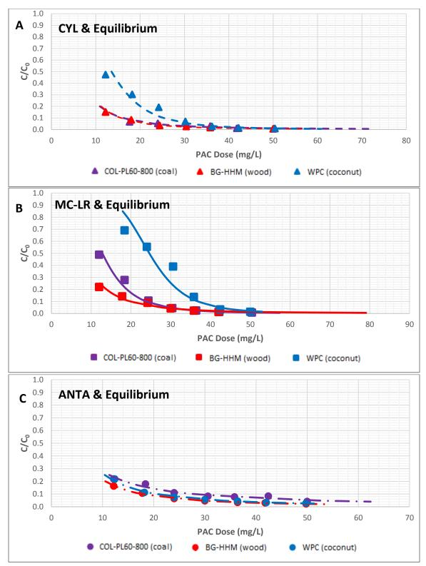
Figure B.76 Cyanotoxin adsorption in the presence of NOM in Lake Erie water using coal-, wood-, and coconut-based PACs, based on the equilibrium data. A) CYL adsorption, B) MC-LR adsorption, C) ANTA adsorption
