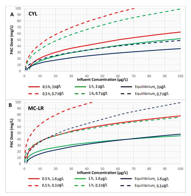
Figure 4.11 Evaluation of the effect of initial cyanotoxin concentration and PAC contact time on BG-HHM dose for CYL and MC-LR adsorption. A) CYL adsorption with initial concentrations of 0.7  $\mu$ g/L and 3  $\mu$ g/L at 0.5 h, 1 h, and equilibrium, and B) MC-LR adsorption at initial concentrations of 0.3  $\mu$ g/L and 1.6  $\mu$ g/L at 0.5 h, 1 h, and equilibrium
