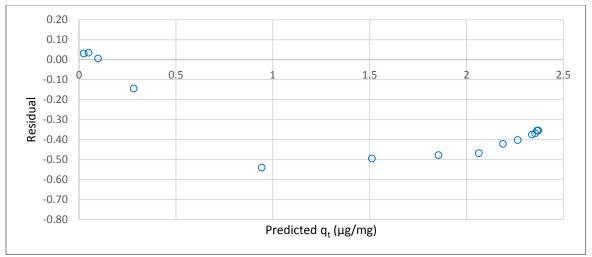
Figure C.8 Residual plot for pseudo-first order fit of CYL adsorption by the virgin Aqua Carb (coconut)
