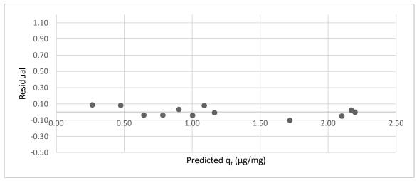
Figure B.7 Residual plot for pseudo-second order fit of MC-LR adsorption by the WPC (coconut)
