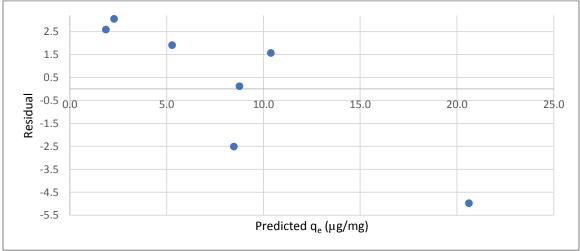
Figure B.23 Residual plot for the equilibrium isotherm of CYL adsorption by the COL-PL60-800 (coal)
