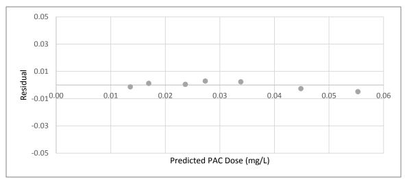
Figure B.55 Residual plot for 0.5 h SEBCM fitting of CYL adsorption by the WPC (coconut)
