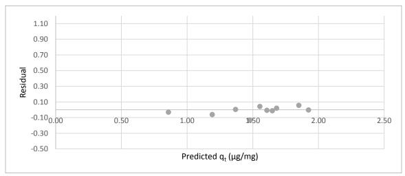
Figure B.4 Residual plot for pseudo-second order fit of CYL adsorption by the WPC (coconut)
