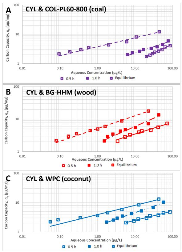
Figure A.49 Freundlich model plot demonstrating PAC adsorption of CYL at contact time of 0.5 h, 1 h and equilibrium (straight lines showing Freundlich fitting curves and symbols showing experimental data). A) Coal-based PAC; B) wood-based PAC; C) coconut-based PAC.
