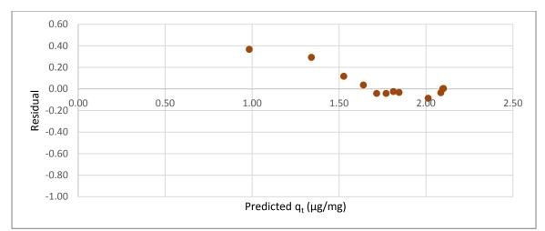
Figure A.19 Residual plot for pseudo-second order fit of ANTA adsorption by the BG-HHM (wood)
