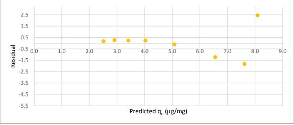
Figure B.32 Residual plot for the equilibrium isotherm of MC-LR adsorption by the COL-PL60-800 (coal)
