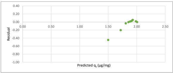
Figure A.17 Residual plot for pseudo-second order fit of MC-LR adsorption by the WPC (coconut)
