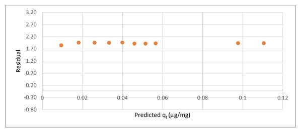
Figure B.13 Residual plot for pseudo-first order fit of CYL adsorption by the BG-HHM (wood)
