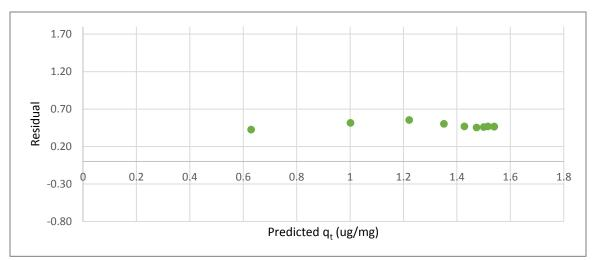
Figure A.7 Residual plot for pseudo-first order fit of MC-LR adsorption by the WPC (coconut)
