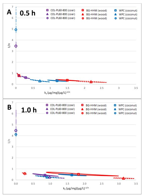
Figure A.48 95% joint confidence regions (ellipse in figures) and point of estimates (points in figures) for the Freundlich parameters of non-equilibrium isotherms generated with the adsorption of CYL, MC-LR and ANTA using the selected PACs in ultrapure water. A) 0.5 h, B) 1 h.
