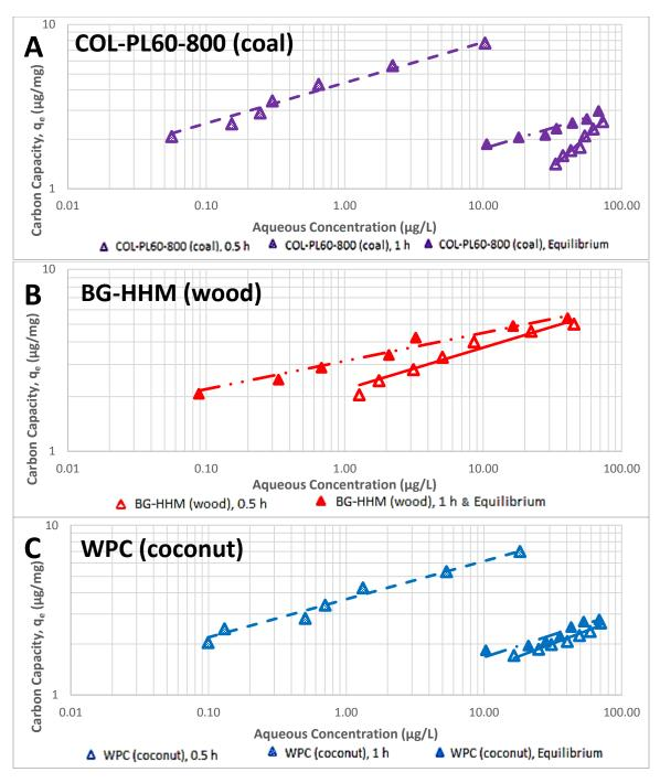
Figure 3.5 Freundlich model plot demonstrating PAC adsorption of MC-LR at contact times of 0.5 h, 1 h and equilibrium. A) coal-based PAC; B) wood-based PAC; C) coconut-based PAC (Straight lines represent Freundlich isotherm model fitting curves and symbols represent experimental data) (In terms of MC-LR adsorption, the wood-based BG-HHM reached equilibrium in about 1 h)
