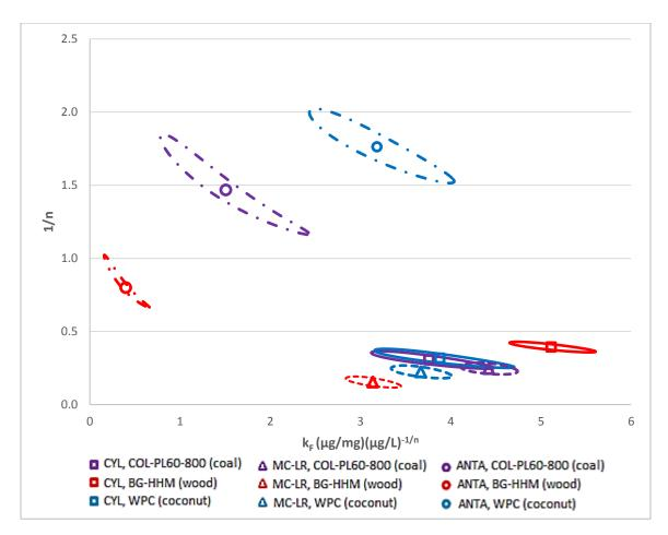
Figure 3.2 95% joint confidence regions and point estimates of the Freundlich isotherm parameters of for the adsorption of CYL, MC-LR and ANTA onto the selected PACs in ultrapure water at equilibrium (Ellipses represent JCRs; symbols positioned in the centre of each ellipse represent the point estimates)
