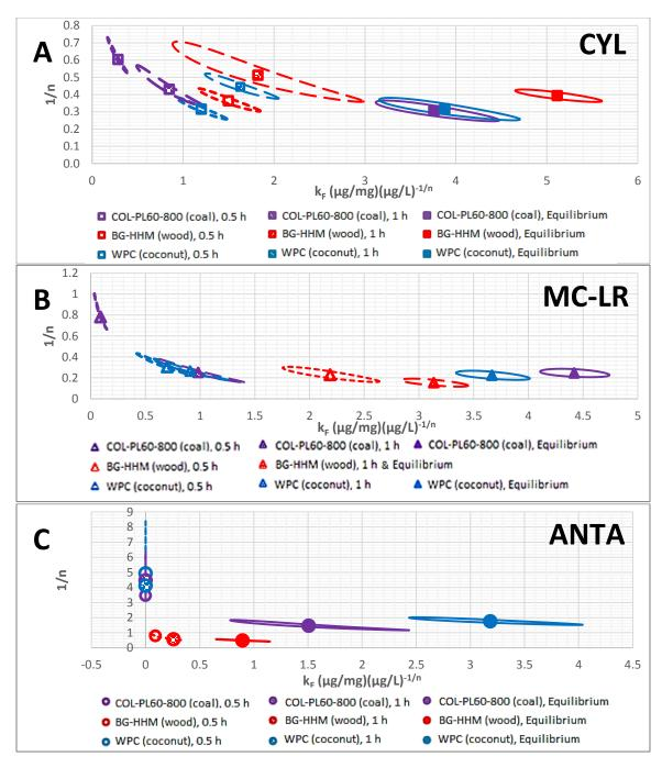
Figure 3.4 95% JCRs and point estimates for the Freundlich parameters of non-equilibrium isotherms generated with the adsorption of CYL, MC-LR, and ANTA using the selected PACs in ultrapure water: A) CYL, B) MC-LR, and C) ANTA (Ellipse curves represent JCRs and symbols in the centre of ellipses represent point estimates) (In terms of MC-LR adsorption, the wood-based BG-HHM reached equilibrium in about 1 h)
