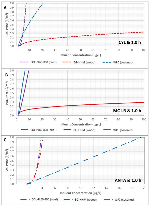
Figure B.74 Estimate of PAC costs for adsorption of cyanotoxins at influent concentrations in Lake Erie water, based on SEBCM under 1 h non-equilibrium conditions, given target cyanotoxin concentration of 1.5  $\mu$ g/L. A) CYL adsorption, B) MC-LR adsorption, C) ANTA adsorption
