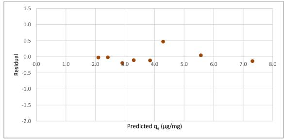
Figure A.44 Residual plot for equilibrium isotherm of ANTA adsorption by the BG-HHM (wood)
