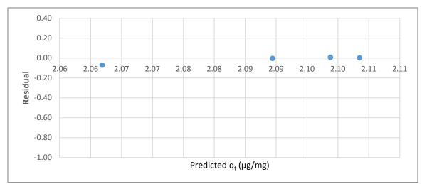
Figure A.16 Residual plot for pseudo-second order fit of MC-LR adsorption by the BG-HHM (wood)
