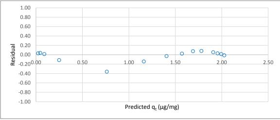
Figure C.3 Residual plot for pseudo-second order fit of CYL adsorption by the virgin Aqua Carb (coconut)
