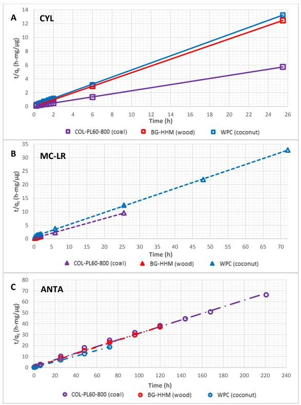
Figure B.1 Pseudo-second order kinetic model fits of CYL, MC-LR, and ANTA adsorption using coal-, wood-, and coconut-based PAC in Lake Erie Water: A) CYL adsorption, B) MC-LR adsorption, and C) ANTA adsorption.
