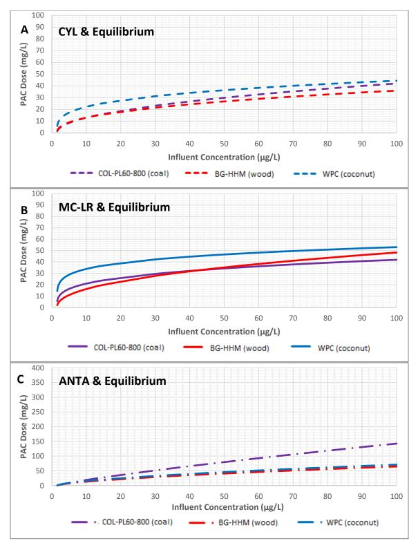
Figure B.77 Estimates of PAC dose for coal-, wood-, and coconut-based PACs for adsorption of A) CYL, B) MC-LR, and C) ANTA adsorption in Lake Erie water, based on SEBCM under equilibrium condition, given target concentration of  $1.5 \ \mu g/L$
