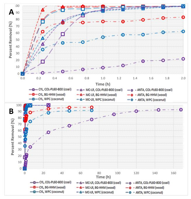
Figure 3.1 Percent removal of CYL, MC-LR and ANTA as a function of time in buffered ultrapure water (pH 7); 100  $\mu$ g/L initial cyanotoxin concentration, 50 mg/L PAC dose. A) 2 h exposure; B) 170 h exposure.
