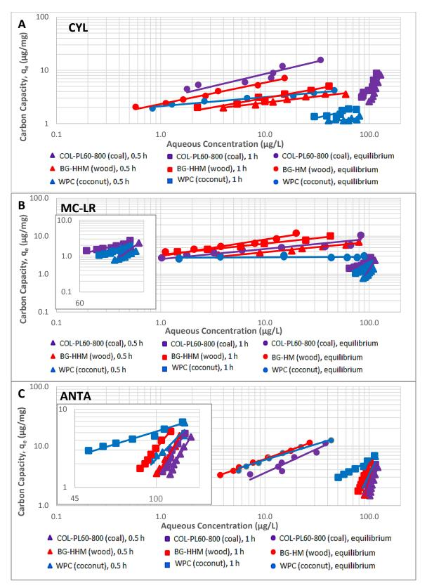
Figure 4.5 Comparison of Freundlich model fitting for three selected PACs at 0.5 h, 1 h, and equilibrium. A) CYL adsorption, B) MC-LR adsorption, and C) ANTA adsorption
