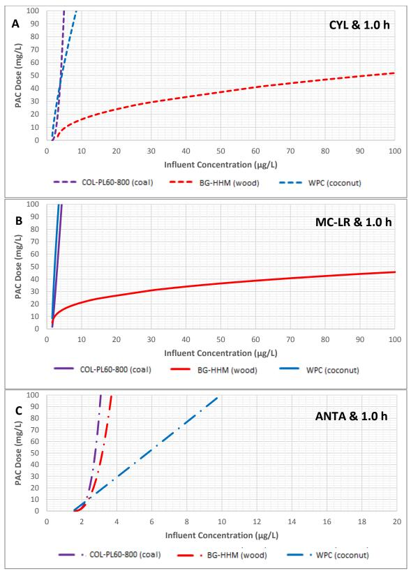
Figure B.73 Estimates of PAC dose for coal-, wood-, and coconut-based PACs for adsorption of A) CYL, B) MC-LR, and C) ANTA adsorption in Lake Erie water, based on SEBCM under 1 h non-equilibrium condition, given target concentration of  $1.5 \ \mu g/L$
