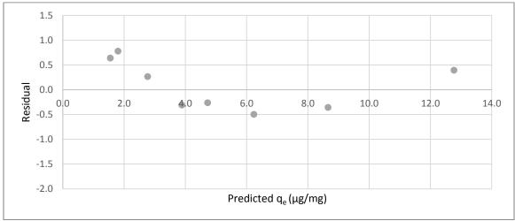
Figure A.29 Residual plot for equilibrium isotherm of CYL adsorption by the WPC (coconut)
