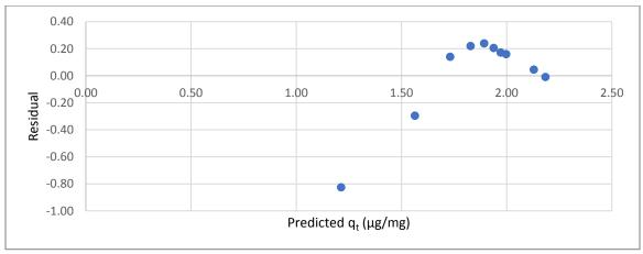
Figure A.12 Residual plot for pseudo-second order fit of CYL adsorption by the COL-PL60-800 (coal)
