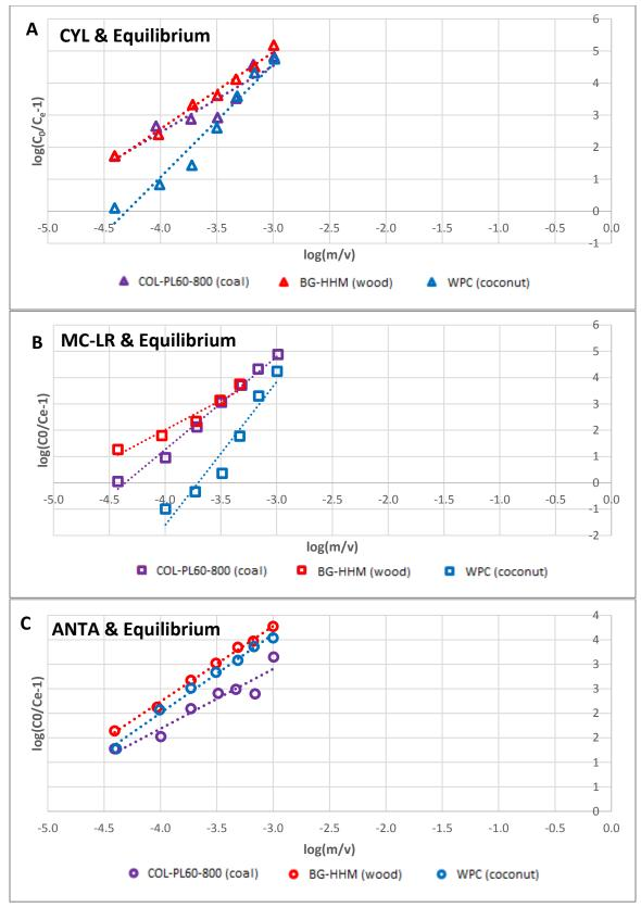
Figure B.75 SEBCM model fitting on the equilibrium carbon loading data for the adsorption of A) CYL, B) MC-LR, and C) ANTA in Lake Erie water
