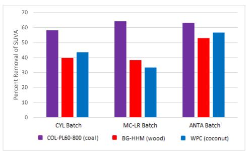
Figure B.80 Percent Reduction of SUVA after adsorption experiment
