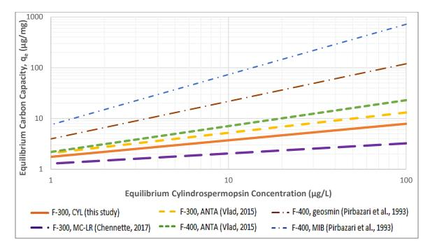
Figure 5.5 Comparison of Freundlich isotherms for CYL, ANTA, MC-LR, MIB, and geosmin by virgin coal-based GACs in ultrapure water. CYL isotherms were prepared using data from the current study, and ANTA, MC-LR, MIB and geosmin isotherms were plot based on the Freundlich parameters obtained from the literature using equilibrium CYL concentrations in the current study, F-300 & F-400 ANTA from Vlad (2015); F-300 MC-LR from Chennette (2017); F-400 geosmin and MIB from Pirbazari et al. (1993).
