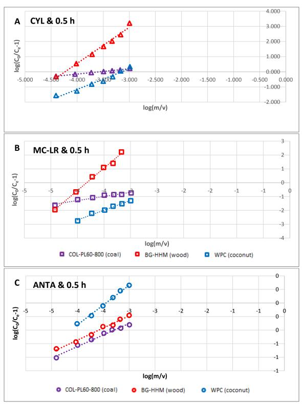
Figure B.52 SEBCM model fitting using the 0.5 h carbon loading data for the adsorption of A) CYL, B) MC-LR, and C) ANTA in Lake Erie water
