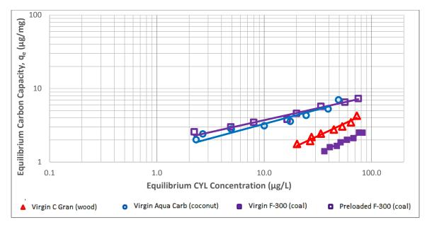
Figure 5.4 CYL Freundlich isotherms for virgin and preloaded GACs in ultrapure water (symbols represent experimental data and straight lines represent Freundlich isotherm fitting curves)
