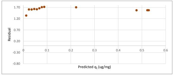
Figure A.9 Residual plot for pseudo-first order fit of ANTA adsorption by the BG-HHM (wood)
