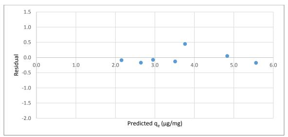
Figure A.34 Residual plot for 1.0 h isotherm of MC-LR adsorption by the BG-HHM (wood)
