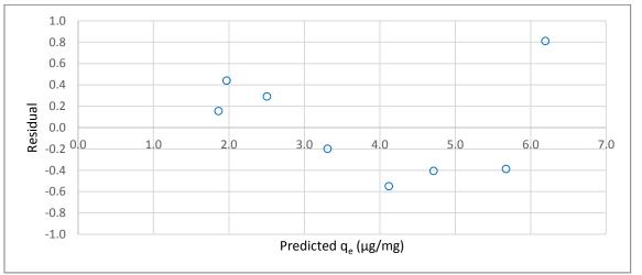
Figure C.12 Residual plot for Freundlich isotherm fitting of CYL adsorption by the virgin Aqua Carb (coconut)
