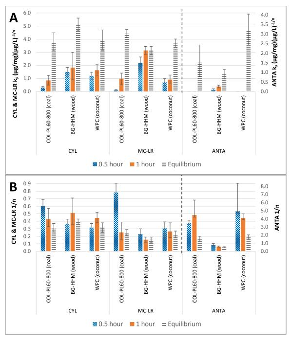
Figure 3.6 Freundlich adsorption parameters (A) K<sub>F</sub> and (B) 1/n non-linear fit with 95% confidence intervals (actual values presented in Appendix A.4)
