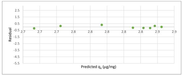
Figure B.38 Residual plot for the equilibrium isotherm of MC-LR adsorption by the WPC (coconut)
