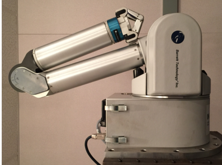
Figure 3.10: Experimental setup of the 4-DoF WAM robot
