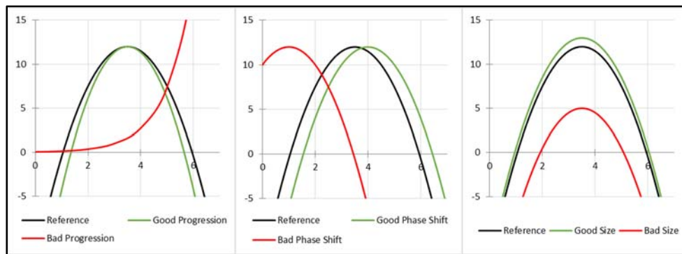
Figure 38. Examples of good and bad progression, phase shift, and size in CORA software
