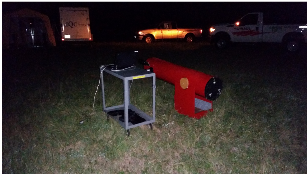
Figure C.9: The calibration telescope at the ground station used to make sure the bacons and quantum signal were collinear. The telescope was setup \approx 20 m away and a visible laser was sent from the transmitter and one beacon at a time for alignment.
