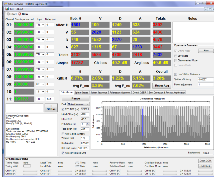
Figure 6.8: A screen-shot of the QKD software developed in the Quantum Photonics Laboratory by Brendon Higgins, Nick Gigov, and Chris Erven. The counts are monitored for each state and the QBER and loss are also measured and displayed. The histogram in the bottom right displays the algorithm searching for the correct peaks between Alice’s and Bob’s time-tags. The blue peak shows the correct alignment has been found for the one second frame of data.
