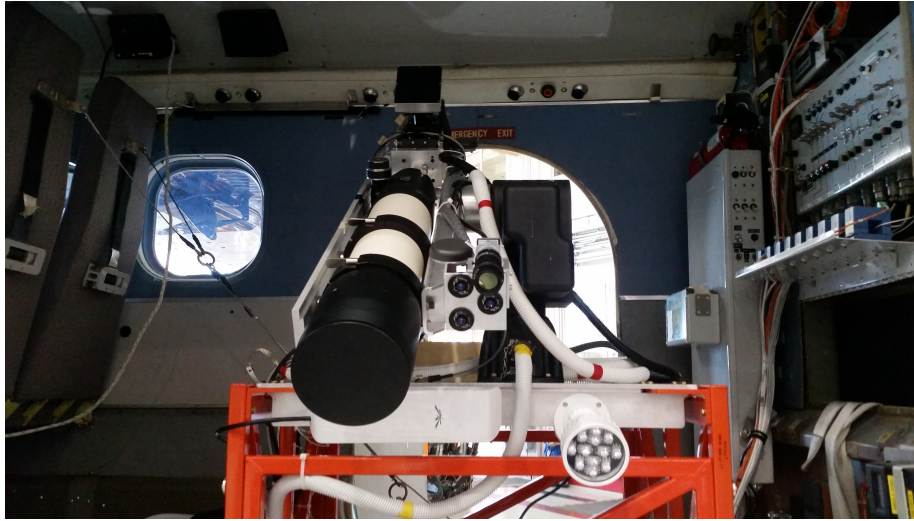
Figure 5.8: Receiver apparatus facing out the port-side door of the NRC Twin Otter research aircraft, showing (clockwise) the telescope, beacon assembly, motor mount, IRL, WiFi antenna, and fine pointing controller (FPC) (behind).
