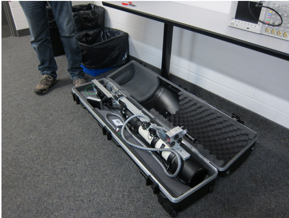
Figure C.3: Carrying case for the QKD receiver telescope, FPU and IOA. We lined a golf club hard travel case with foam to secure the receiver in place when the lid was closed. The case had wheels which allowed for easy transport.
