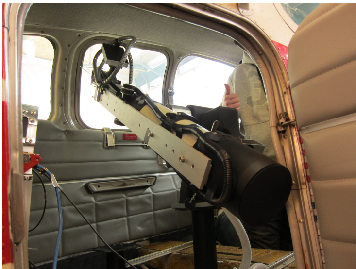
Figure 4.6: The receiver telescope mounted into the Beechcraft Bonanza airplane. The telescope looks out the rear baggage compartment door, and has a small angular sweep of approximately 10^\circ because the rear of the telescope hits the window on the other side. The front of the electronics crate can also be seen towards the left of the photo.
