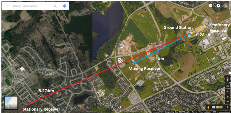
Figure 4.7: The two sites for the local tests of the equipment developed for the QKD receiver. The truck drove along a road approximately 1.21 km away from the ground station and a stationary site was chosen approximately 3.27 km from the ground station. Imagery and map data ©2017 Google.
