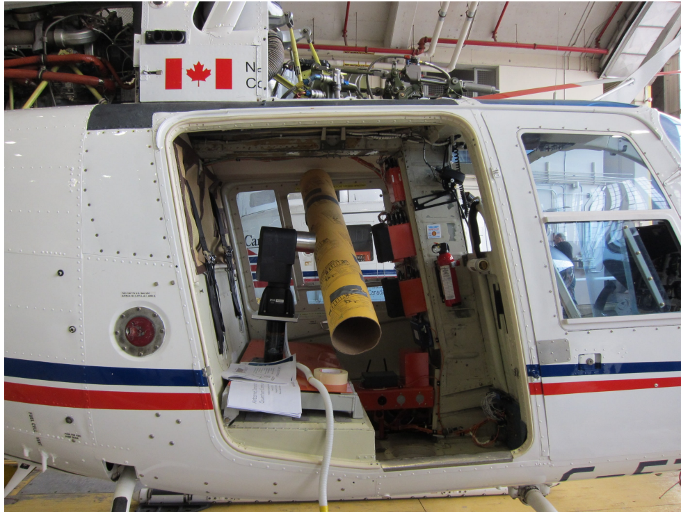
Figure C.5: Fitting the replica receiver telescope and FLIR mount into the Bell 206 helicopter to check ranges of motion. The angular range of the telescope was limited because the back of the telescope came into contact with the back door.
