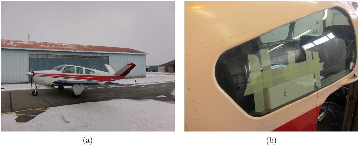
Figure 4.4: (a) The Beechcraft Bonanza airplane used for testing the WiFi equipment planned to be used for the classical link during the QKD trials. (b) The WiFi antenna mounted into the rear window of the airplane.
