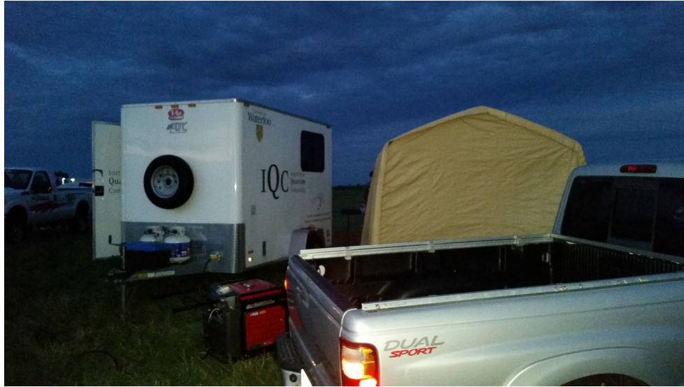
Figure C.8: The IQC trailer setup at the Smiths Falls–Montague Airport along with the generator and tent to protect the transmitter from the elements when the experiment was not in session.
