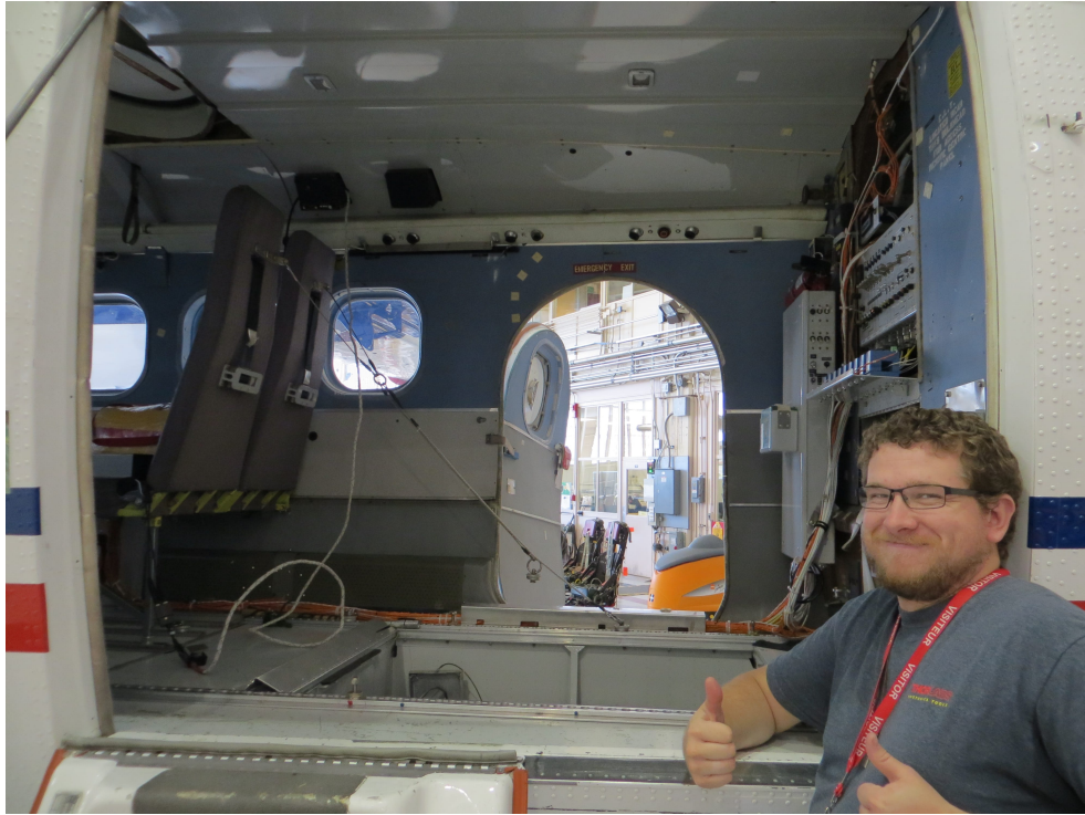
Figure C.14: Preparing the cabin of the airplane to install the QKD receiver telescope and electronics. The port in the bottom of the plane normally holds a camera for other experiments but was closed for our flights.
