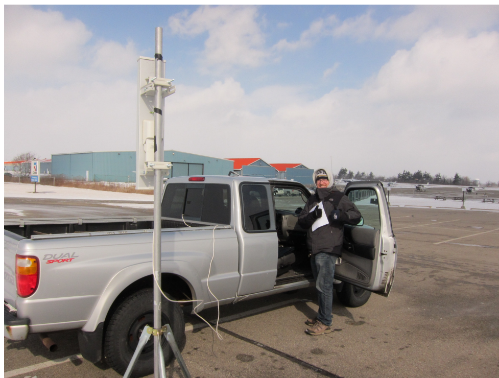
Figure C.1: Testing the WiFi at the Brampton Airport. The WiFi antenna was placed in the back of the truck and rotated to follow the airplane as it flew past. It was very cold and we had to switch WiFi rotators part way through the experiment. An incoming snowstorm halted further distance testing as we could no longer see the airplane and the air was becoming too turbulent for comfortable flight.
