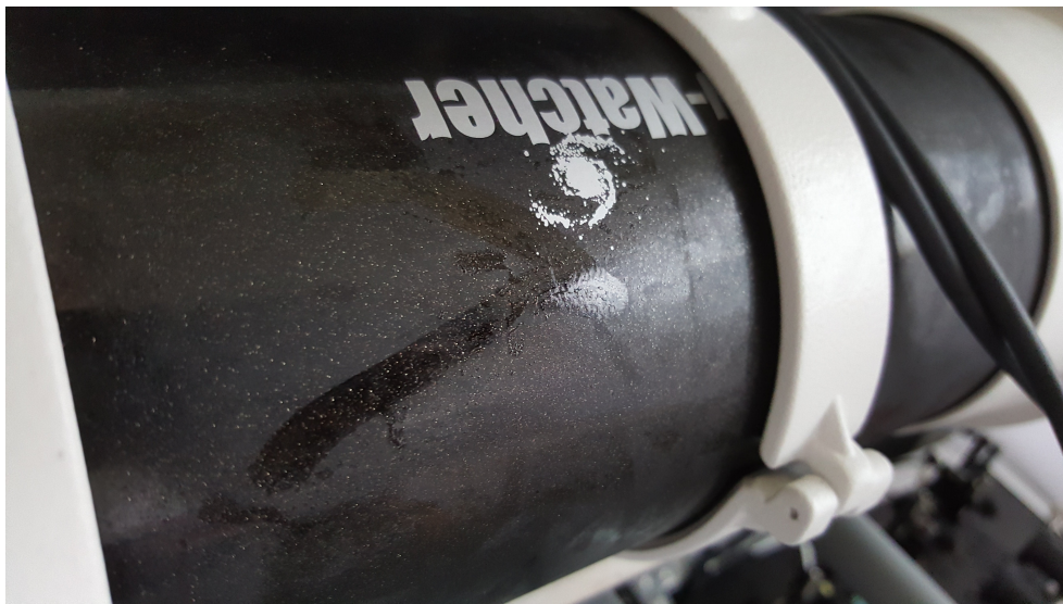
Figure C.11: Dew forming on the transmitter telescope on Monday September 19th, 2016, the day before the first flight.
