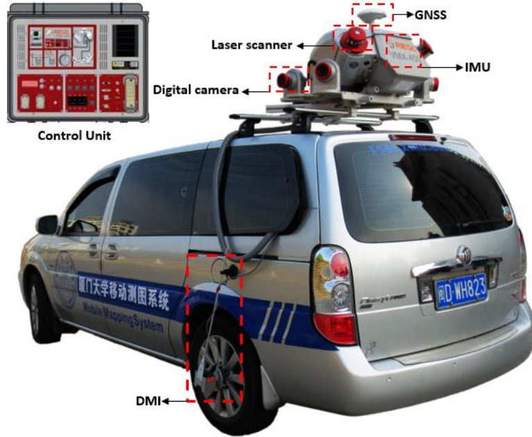
Figure 3.1 System configuration of a RIEGL VMX-450 system.
