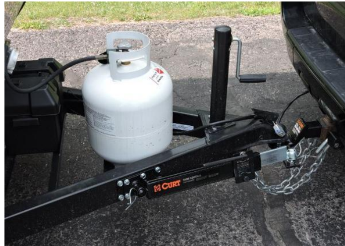
Figure 2.4: Sway control via friction damping element [17]
