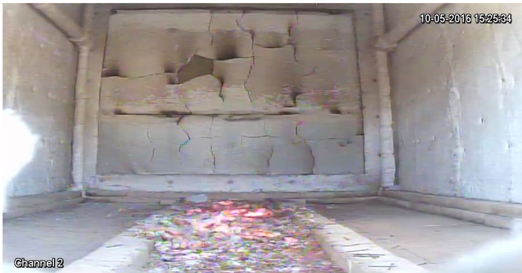
Figure 7.11: Real wall test #1, fire-side camera, 66.1 min.
