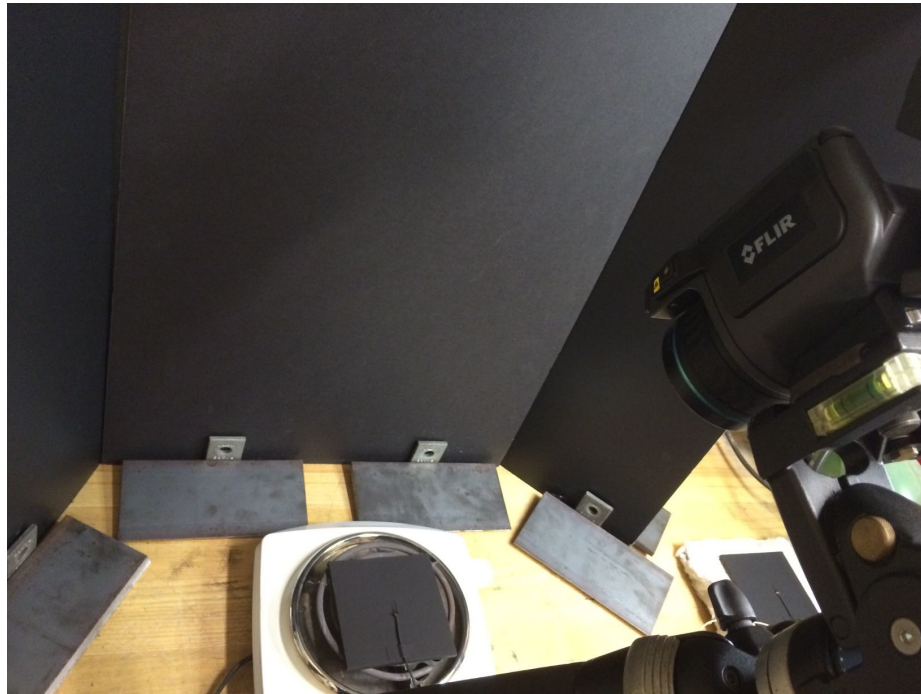
Figure 5.11: Measurement of temperature-dependent emissivity (setup).
