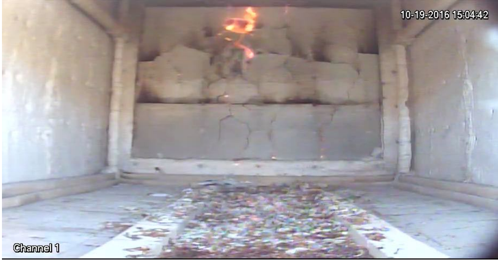
Figure 7.23: Real wall test #2, fire-side camera, 110.3 min.
