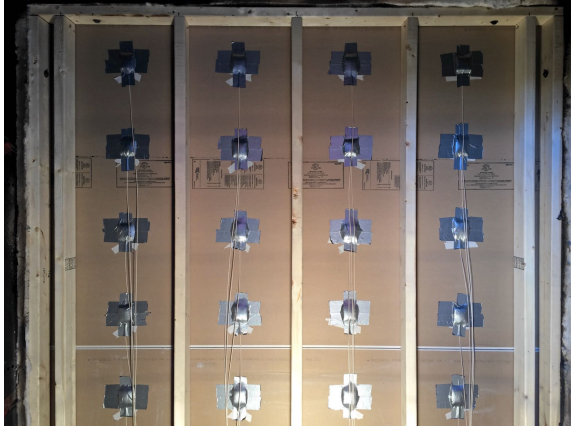
Figure 7.5: In-cavity thermocouples, uninsulated cavities.
