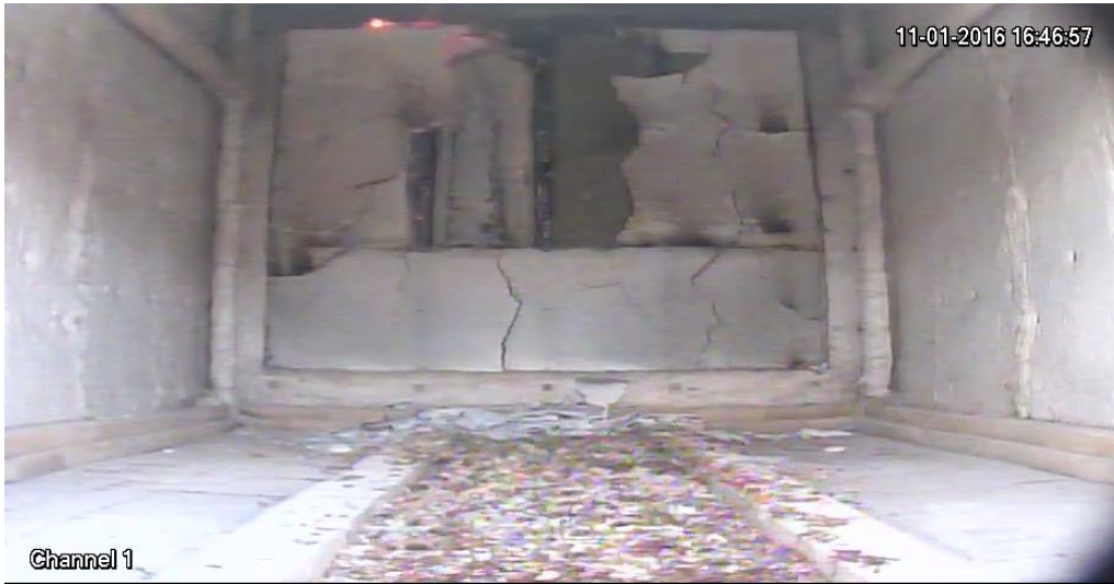
Figure 7.37: Real wall test #4, cool-side camera, 107.8 min.
