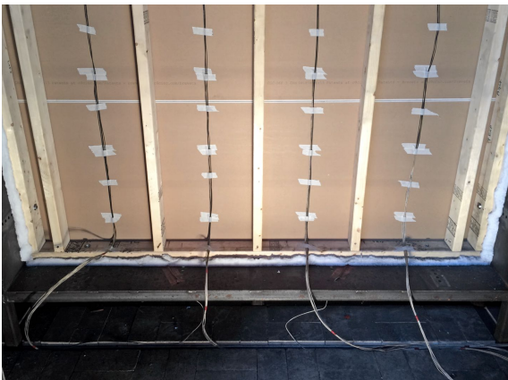
Figure 7.3: In-cavity thermocouples, insulated cavities.
