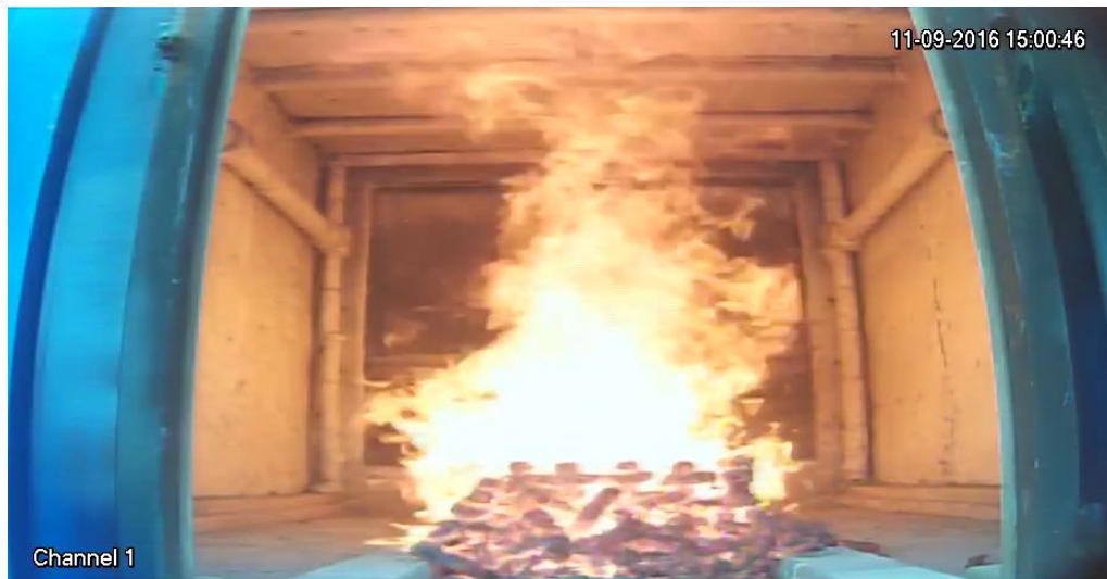
Figure 7.45: Real wall test #5, fire-side camera, 27.1 min.
