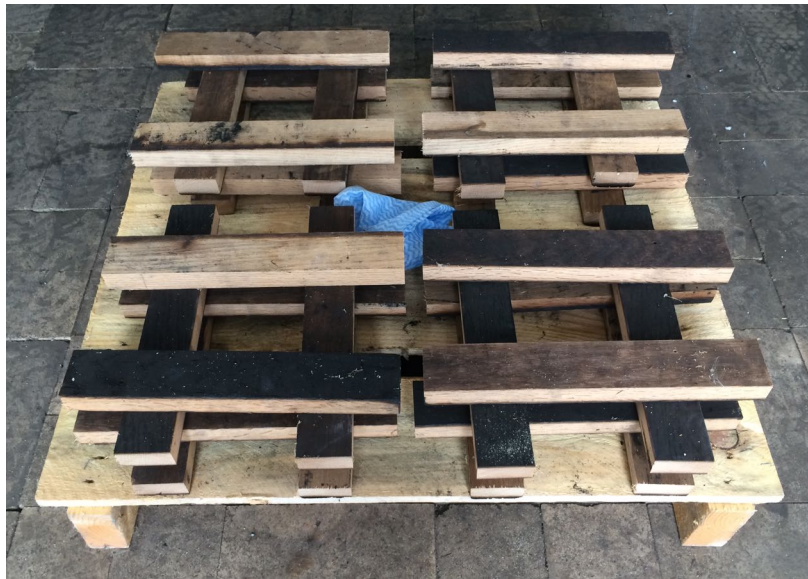
Figure C.8: Fuel contents for characterization test #2.
