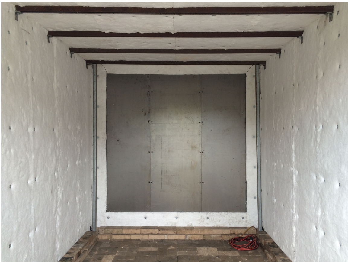
Figure 4.7: Fully insulated fire compartment.
