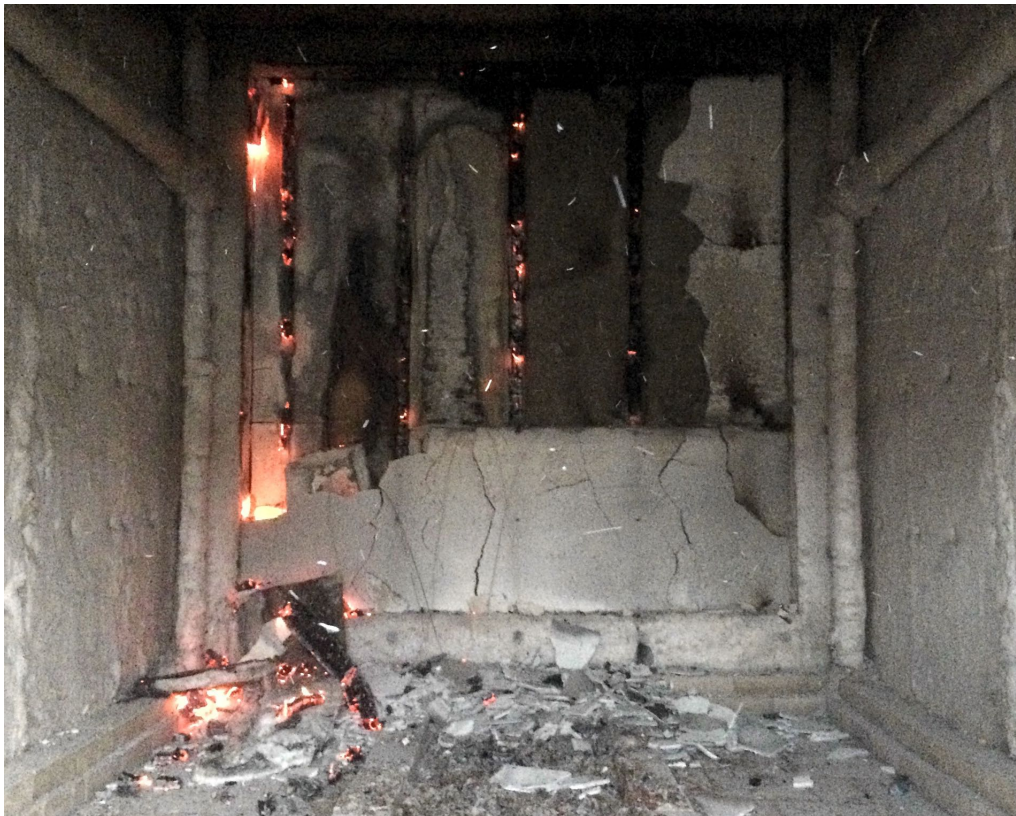
Figure 7.38: Real wall test #4, cool-side camera, end-of-test.
