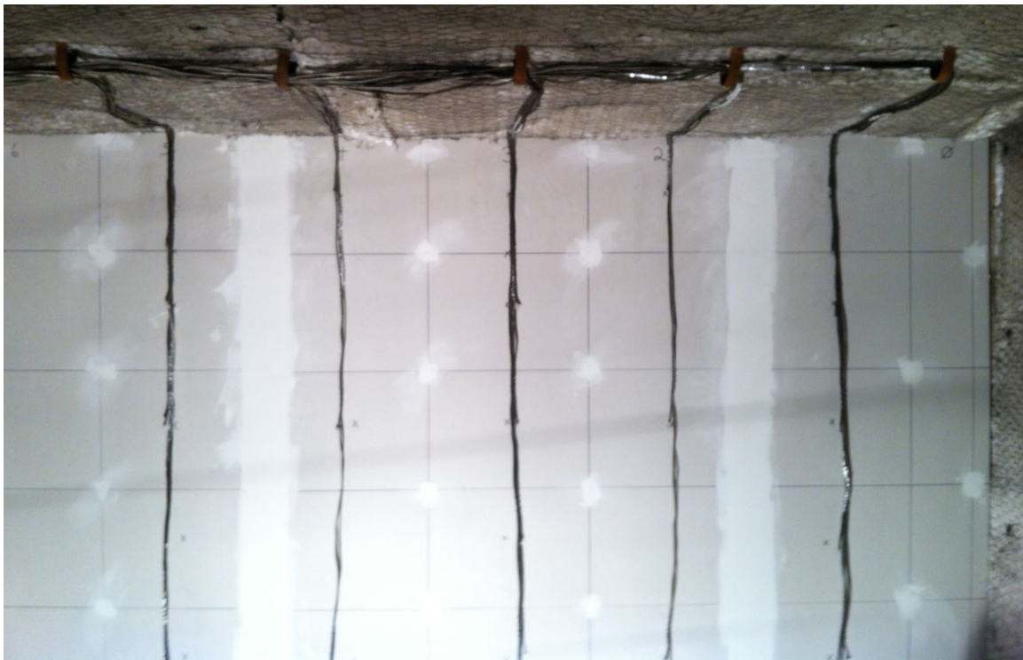
Figure 3.5: Exposed-side thermocouples hanging in front of the test wall.
