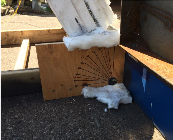
Figure 6.31: Obstruction panel opening angle measurement.
