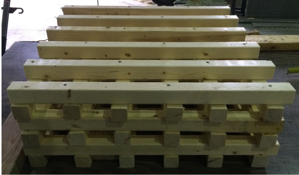
Figure 6.1: Standard wood crib used in the large-scale experiments.
