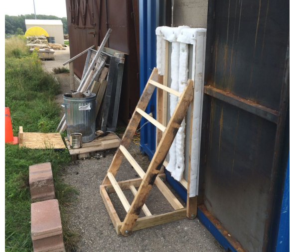
Figure 6.24: Ventilation obstruction panel, fully closed.
