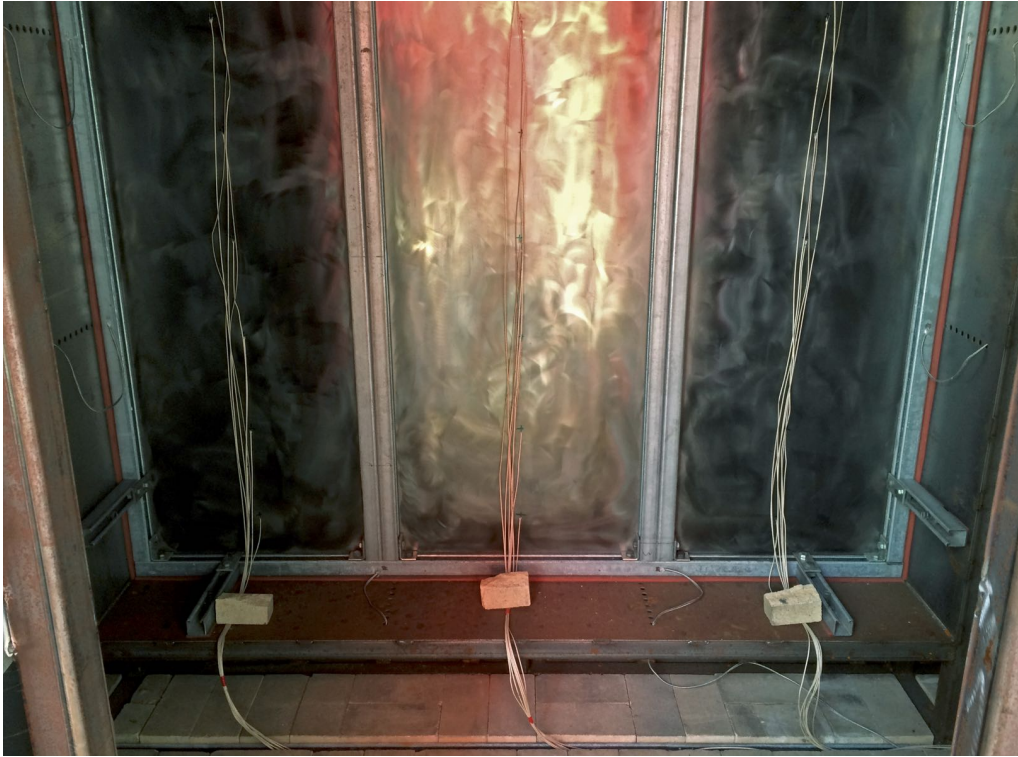
Figure 5.1: Thermocouples installed on the unexposed side of the steel wall.
