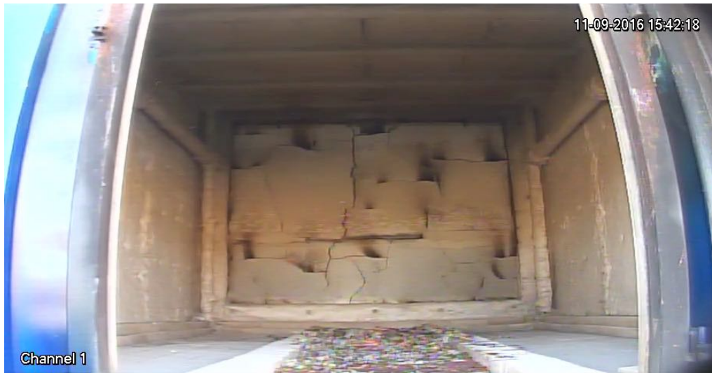
Figure 7.46: Real wall test #5, fire-side camera, 68.2 min.
