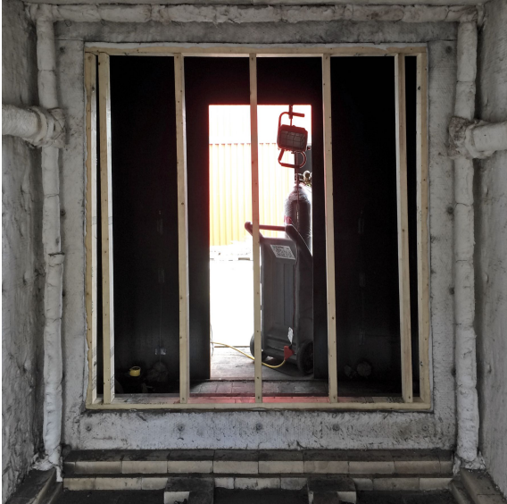
Figure 7.1: Wood stud frame mounted in the fire test apparatus.
