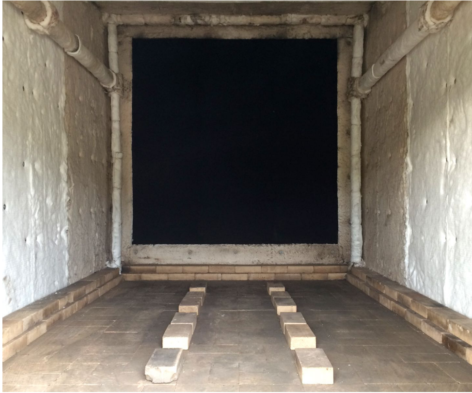
Figure 6.37: Renovated compartment interior following the test #6 structural failure.
