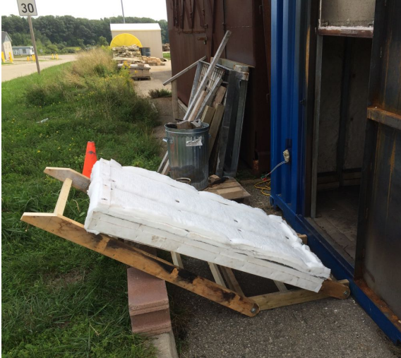
Figure 6.23: Ventilation obstruction panel, fully opened.
