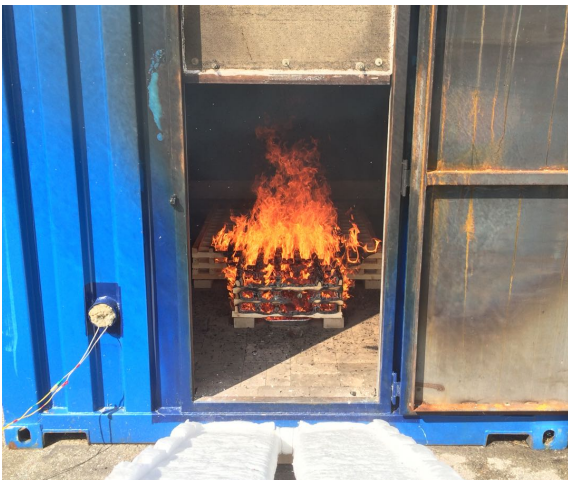
Figure 6.25: Characterization test #5, fire, t = 10 min.
