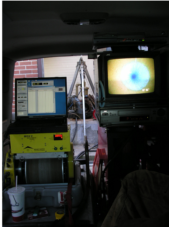
Figure A.11: Monitoring setup for profiling Well 01.
