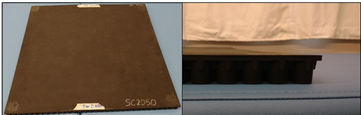
Figure 4.3: The Square sample of SmartCells™ safety flooring used (Left); a cross-section image of the SmartCells™ sample, displaying the rubber columns found underneath the top surface (Right)
