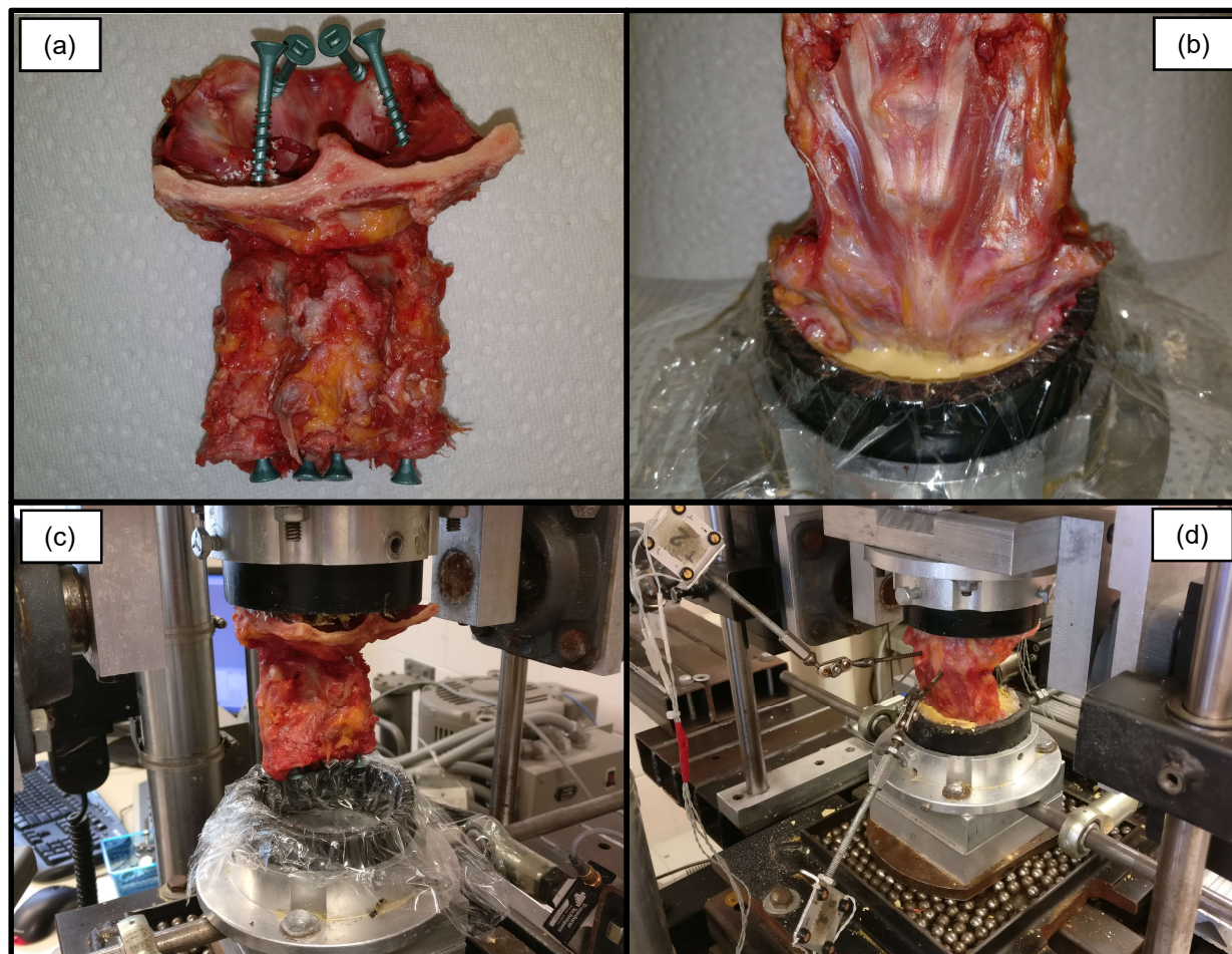
Figure 59: Potting procedure for cadaveric specimens: a) screws placed into C0 and C3 for additional potting strength, b) C0 potted first in dental cement, c) C3 potted second in Instron to ensure proper alignment and d) potted specimen with optical markers attached
