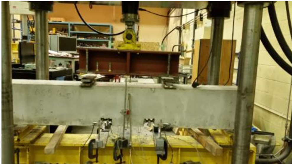
Figure 5.4 Lap splice beam installed in the test frame
