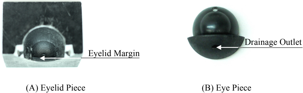
Figure 5-8. Eyelid piece showing the DM eyelid margin (A) and eye piece showing the drainage outlet (B).
