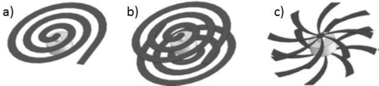
Figure 9: Serpentine structures (a) Basic concept, (b) Double Beam Sandwich, (c) Tethered structure
