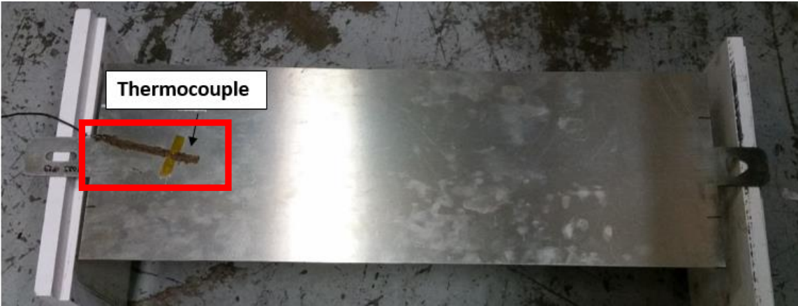
Figure 121: Blank preparation with a thermocouple to determine heating times
