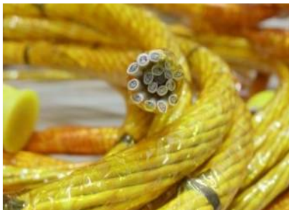
Figure 1.2: Typical cable used in spacecraft, [142].
