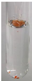
Figure 14. Hydrophobic FpC_3NMe_2 solids float or sink in water.
