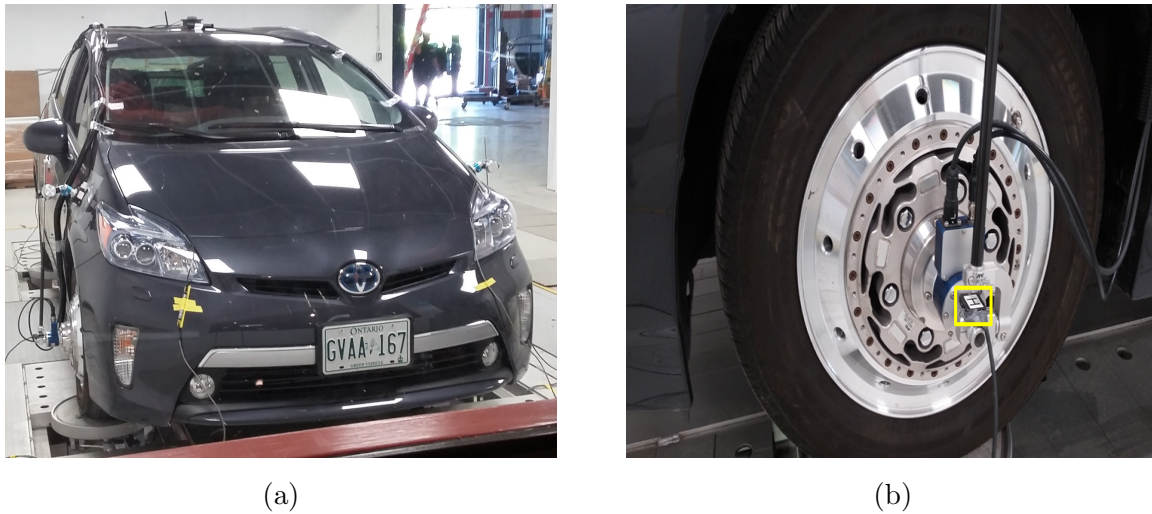
Figure 4.5: 4-Post test rig: (a) Prius on 4-Post rig and (b) Accelerometer attached to the wheel hub
