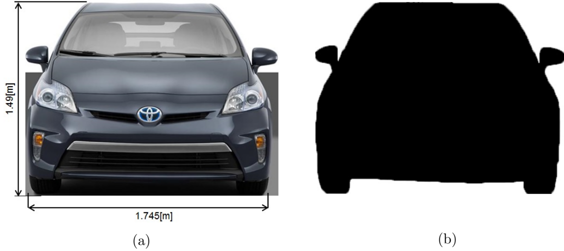
Figure 5.2: Frontal area: (a) Frontal image of Prius and (b) Processed frontal image of Prius to black and white
