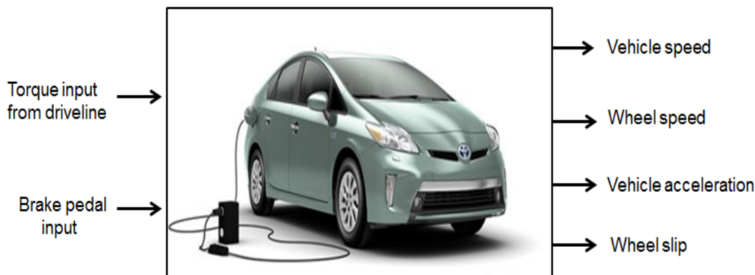
Figure 3.2: Inputs and outputs of the MapleSim model
