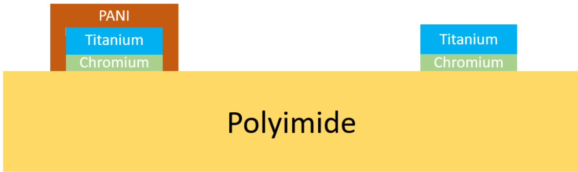
Figure 34. PANI electropolymerized onto the active electrode.
