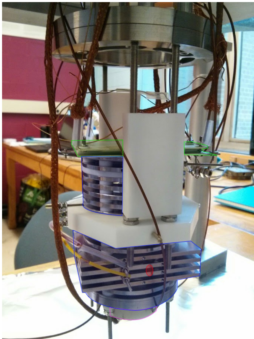
Figure 2.4: Photo of the CEI spectrometer depicted schematically in Figure 2.3 out of its high vacuum chamber. (Green) Cation PSD. (Blue) Concentric rings defining extraction field. (Red) X-ray entrance. (Pink) Electron detector.
