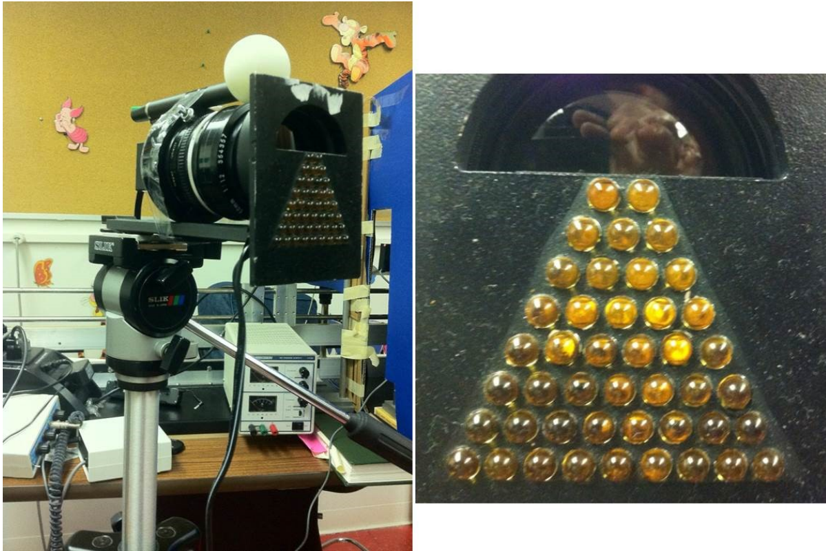
Figure 2-1: Dynamic high speed photorefractor. This image was reprinted from my Master's thesis.
