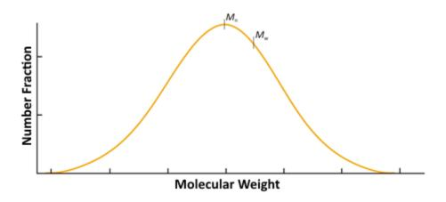
**Figure 2**. Graph illustrating the distribution of molecular weights amongst polymer chains.
