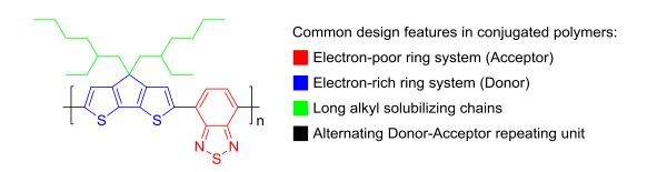
**Figure 1**. Conjugated polymer incorporating common design features.
