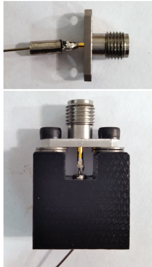
Figure 6.4: The configuration of the connection assembly of the PE SMA wire illustrating the crimping, SubMiniature version A connectors, and Delrin insulating block.
