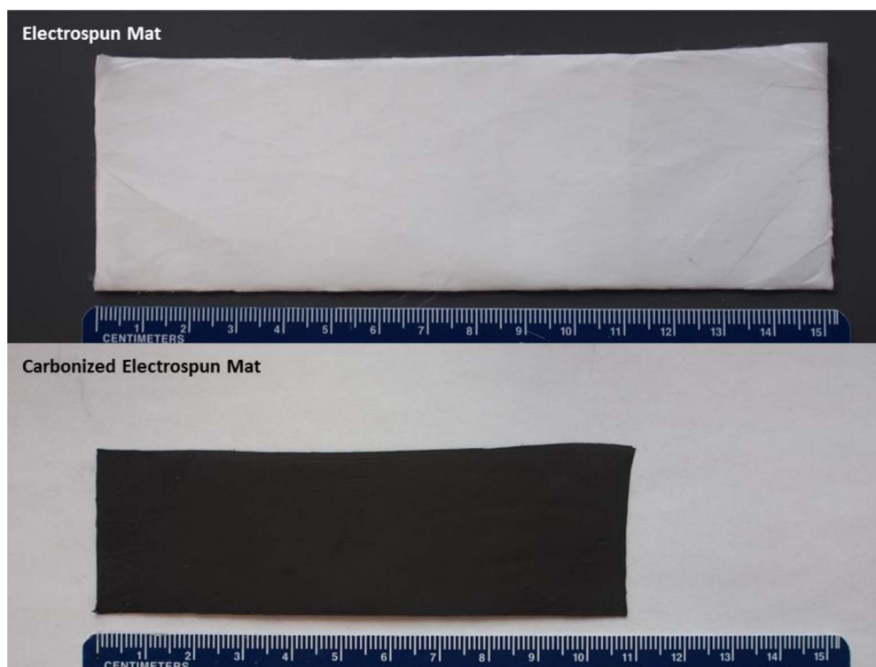
Figure 4. Images of electrospun PAN mat before and after carbonization.
