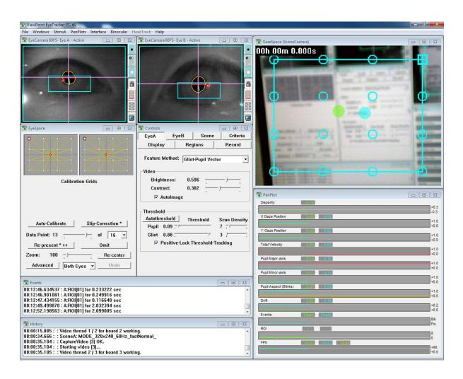
Figure 2.3. The glint-pupil vector method was selected to track eye position. The top left shows Eye A (right eye), and Eye B (left eye). The bottom left is the EyeSpace indicating the calibration grid. The top right was the GazeSpace which was connected to the scene camera. The bottom right was the pen plot where x and y gaze points and velocity were recorded
