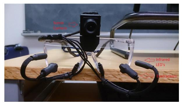
Figure 2.2 Arrington eye tracker. Scene camera located above the nasal bridge; eye tracking cameras and infrared LEDs located in front of each eye
