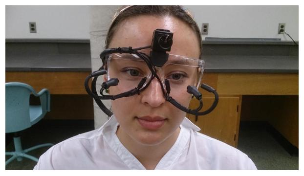
Figure 2.1. Arrington Research Viewpoint Binocular eye tracker mounted. Informed consent was given for the use of this photograph.
