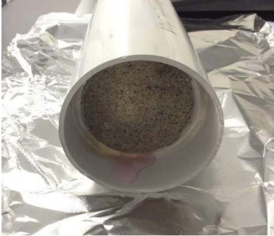
Figure 5 A sandstone core sealed along the axial surface with concrete/masonry silicone, then set into PVC sleeve with silicone near the faces of the cores. The PVC pipe extends slightly beyond the face of the core on both ends.
