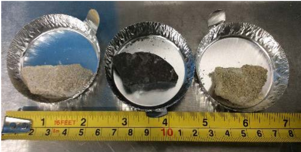
Figure A-1 Example pieces, from left to right, of Indiana carbonate limestone, Mancos shale, and Idaho Gray sandstone.
