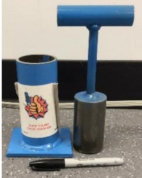
Figure 7 Portable or hand-held steel rock crusher used to crush puck samples for extraction.
