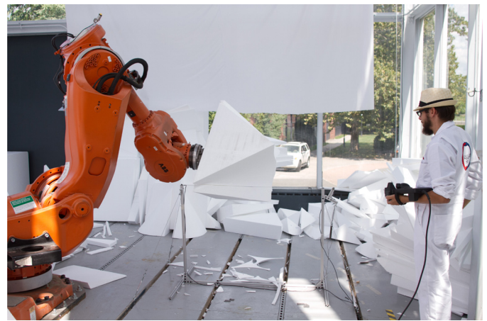
Fig. 3. Operation of the digital fabrication where the parametric models were programmed to output ABB Robot code of cutting paths for the robotic fabrication to generate the foam pieces by having the robot pick up rough cut blocks and then drag the foam through a large hot wire to create specific geometric surfaces.
