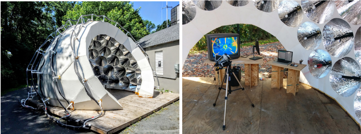
Fig. 8. The Thermoheliadome in its fully functional state with reflective cones and evaporatively cooled supply water circuits. The photo on the right shows a thermal image of a cone during operation on the television screen, demonstrating the apparently uniform cool (blue) surface achieved via reflection. (For interpretation of the references to color in this figure legend, the reader is referred to the web version of this article.)
