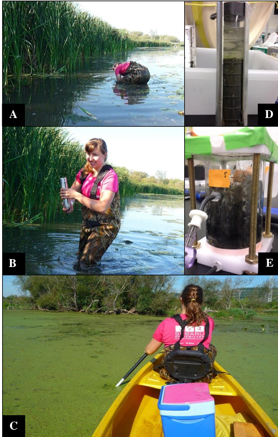
Figure 2.2. Photos of field sampling and sediment core flow through reactors. (A) Sediment cores were collected by crouching in the water and pushing the hand corer into the sediment. (B) A rubber stopper was inserted in the bottom to plug the hand corer and retrieve a sediment core. (C) There was extensive filamentous green algae growth in Cootes' Paradise marsh on the day of sampling. Sediment cores back to the laboratory in a cooler. (D) Sediment cores were collected without disturbing the sediment-water interface. (E) The lining of the hand corer with intact sediment served as the reactor vessel in the sediment core flow through reactors used in the experimental setup.
