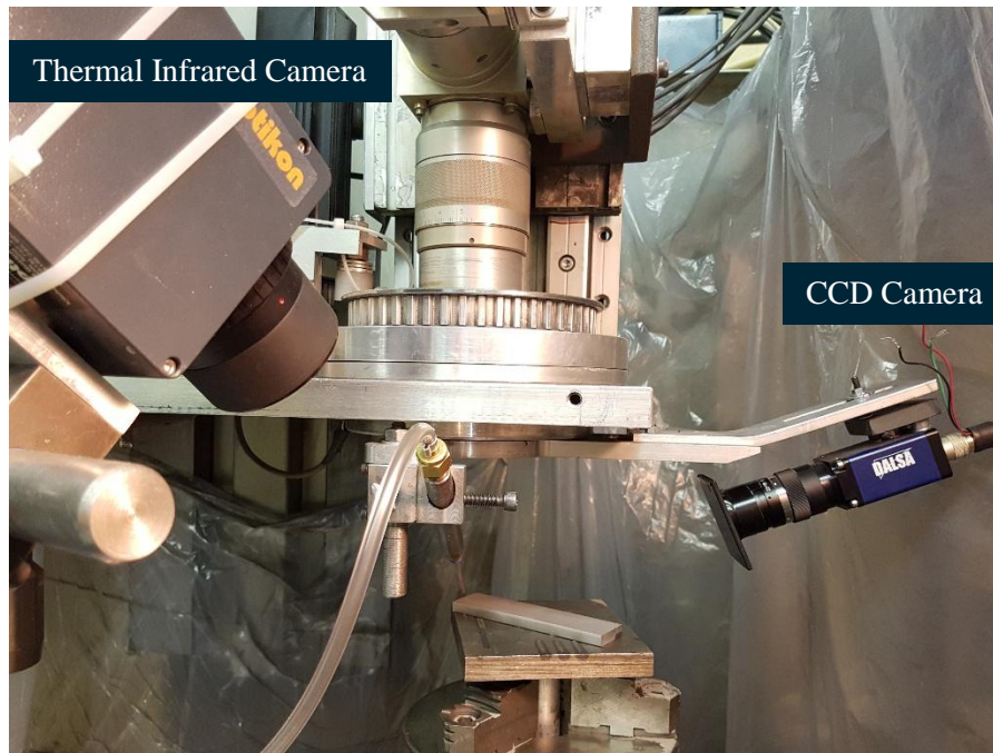
Figure 3-3 Integrated CCD and thermal infrared monitoring of the LMP process.
