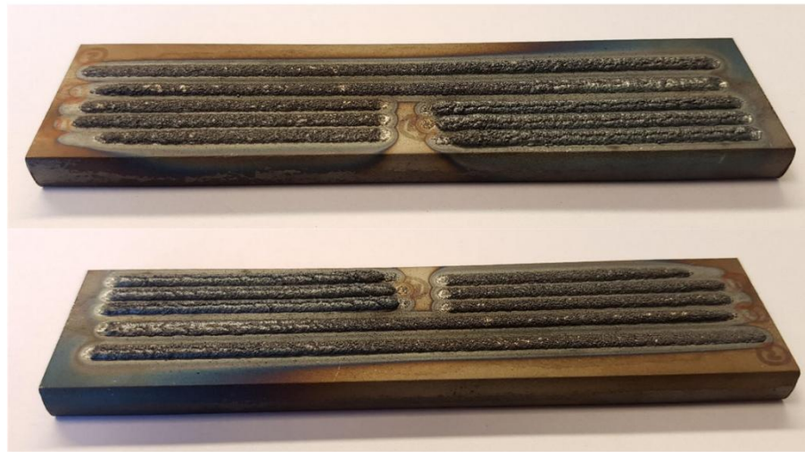
Figure 6-54 Single-track and multi-track LAM samples K1-c and K2-c with closed-loop integrated cooling rate and clad height control.
